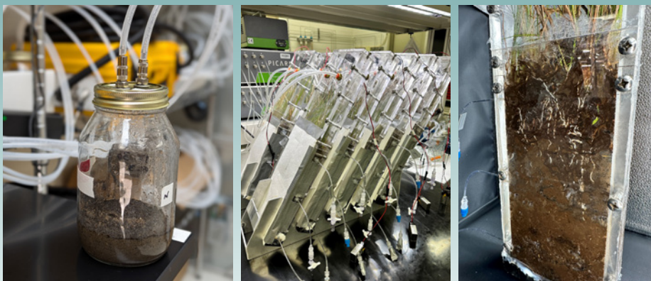
Figure 12. SoilCosms (left photo) allow reproducible, high-throughput experiments with self-guided automation. Arctic mesocosms containing tundra plants and soils (right photos) allow simultaneous porewater sampling and monitoring of root growth and greenhouse gas fluxes.
