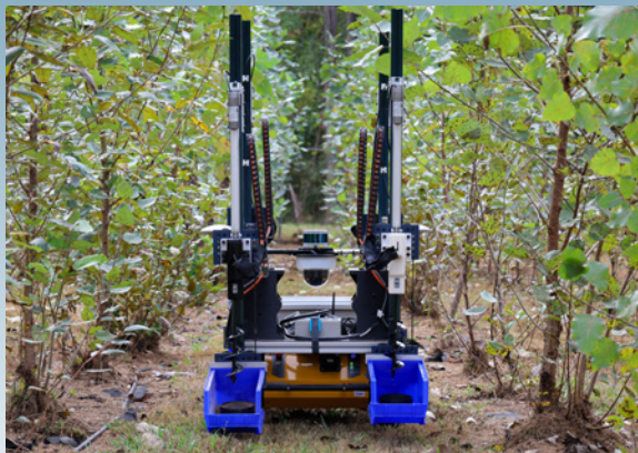
Figure 16. Researchers at the DOE Manufacturing Demonstration Facility at ORNL created this soil sampling robot for the SMART Plant project.
