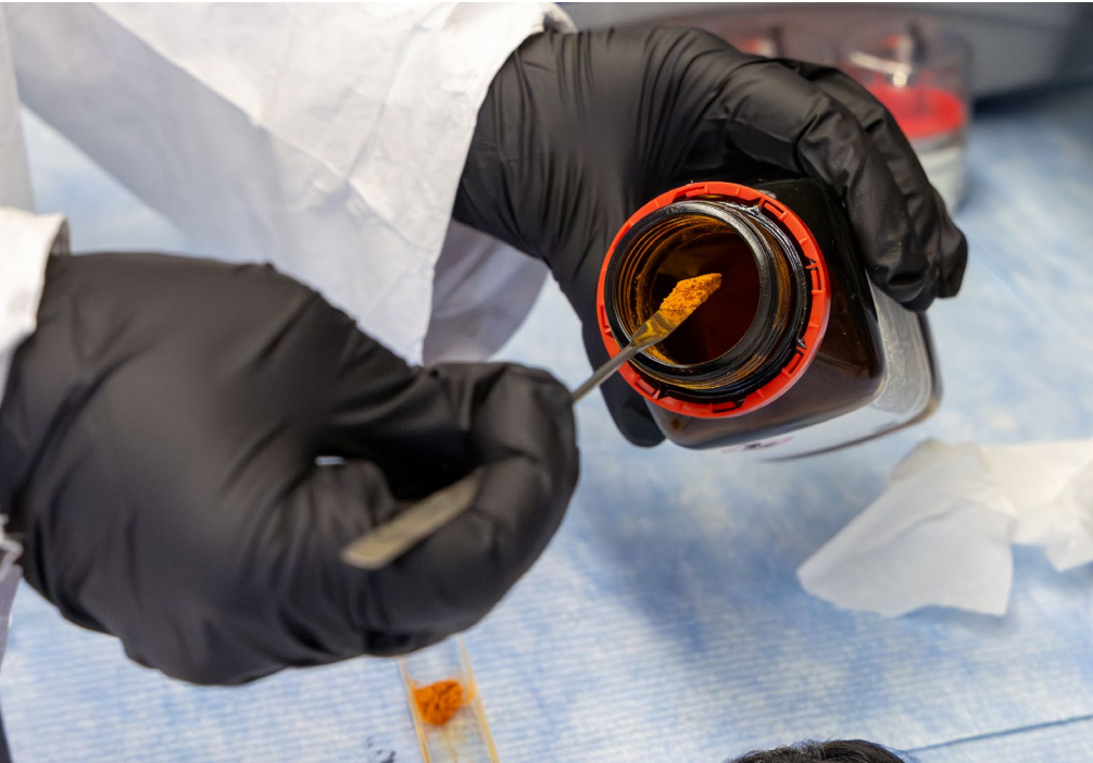
R&D Radiochemist Pavithra Kankanamalage weighs resin to pack a column that will later be used to separate radioisotopes.
