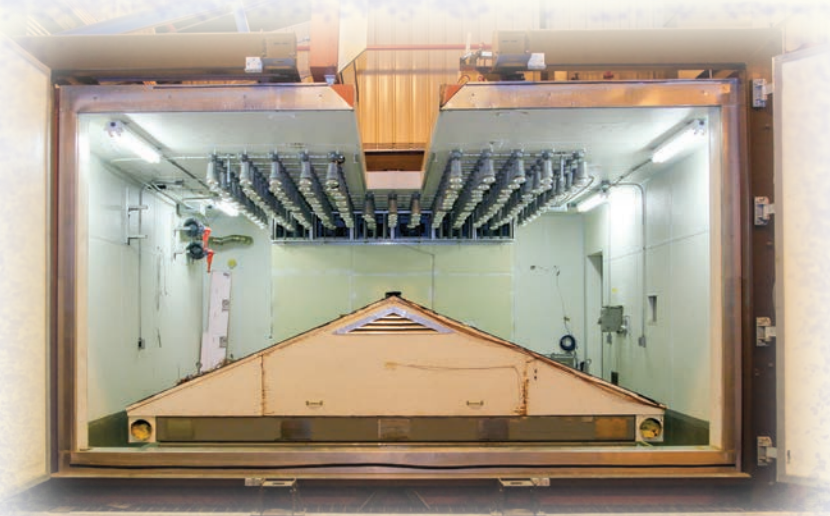
Apparatus for low-sloped roof or roof/attic system performance characterization (Building 3144)
