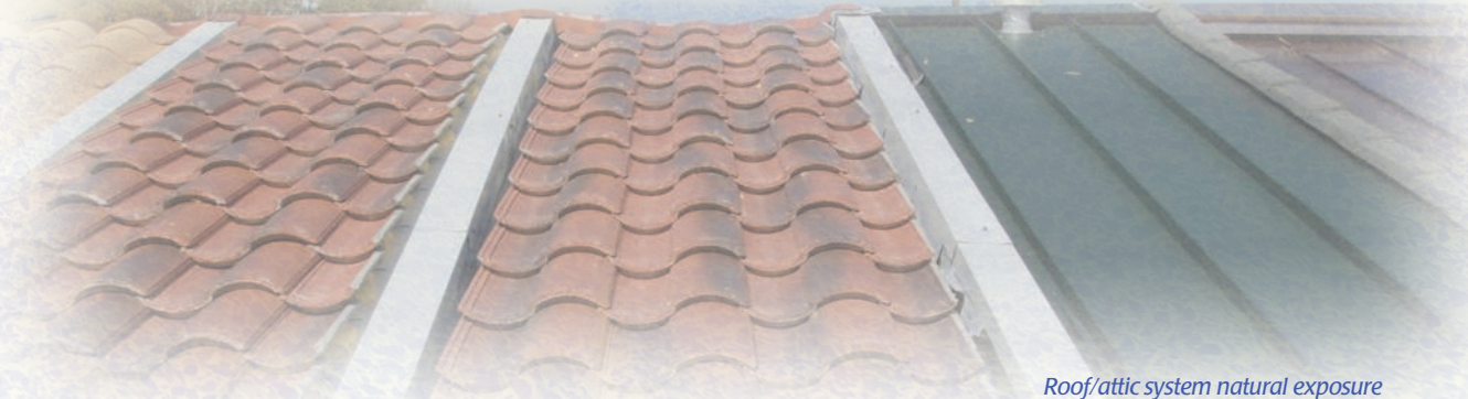
Apparatus for low-sloped roof or roof/attic system performance characterization (Building 3144)
