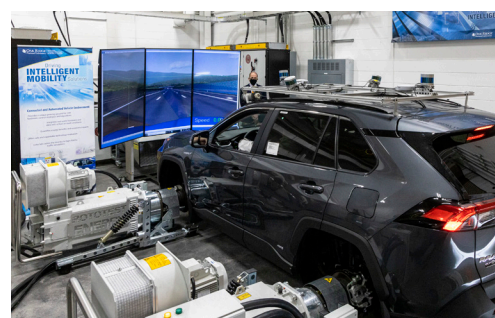
The Connected and Automated Vehicle Environment Laboratory is a unique proving ground to evaluate intelligent mobility solutions using real-world hardware and data in virtual traffic conditions.
