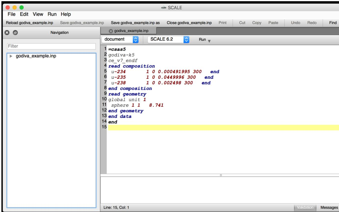
The screenshot displays the SCALE 6.2 software interface. The main window shows a text editor with the following input file content:
