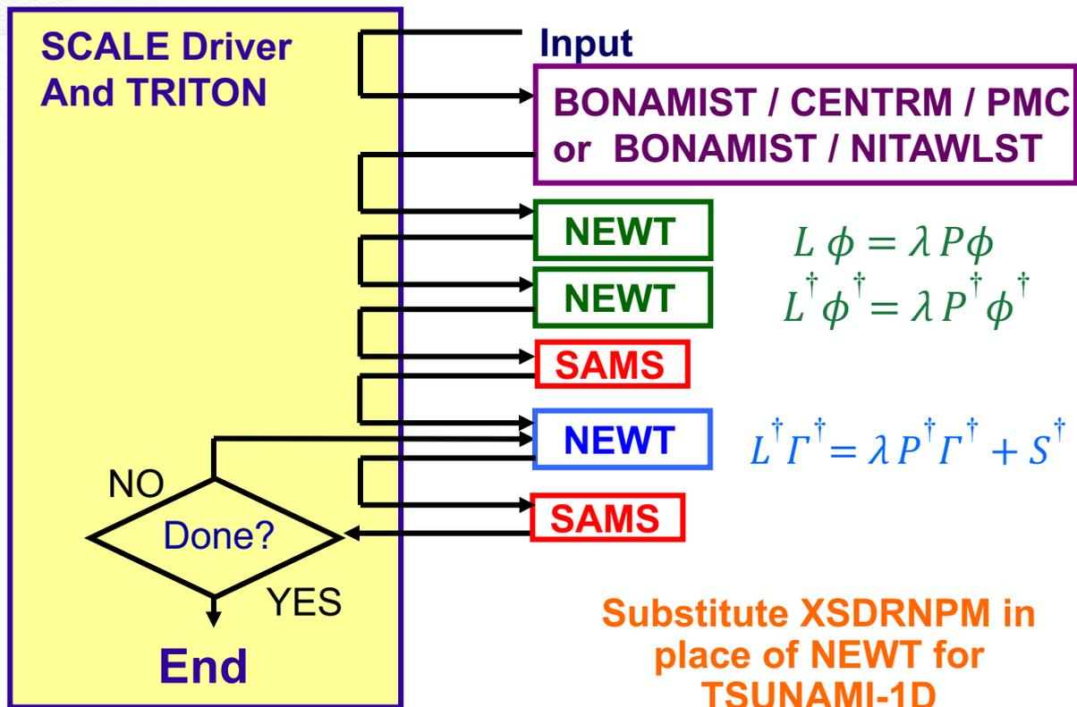
Resonance cross-section processing
