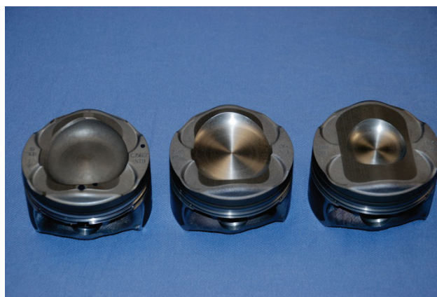
Figure 2. The pistons used in the tests for (left to right) compression ratios of 10.1, 12, and 13.
