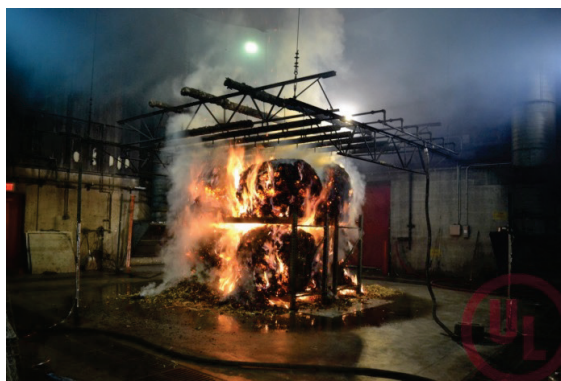
ORNL is working with UL to evaluate how feedstock type, bale shape, and bale spacing affect fire intensity under controlled conditions. (Images courtesy of UL.)
