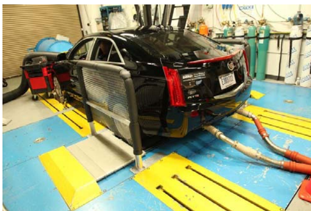
Researchers at the National Transportation Research Center evaluate engine technologies with high-octane fuels using this modified Cadillac ATS.
