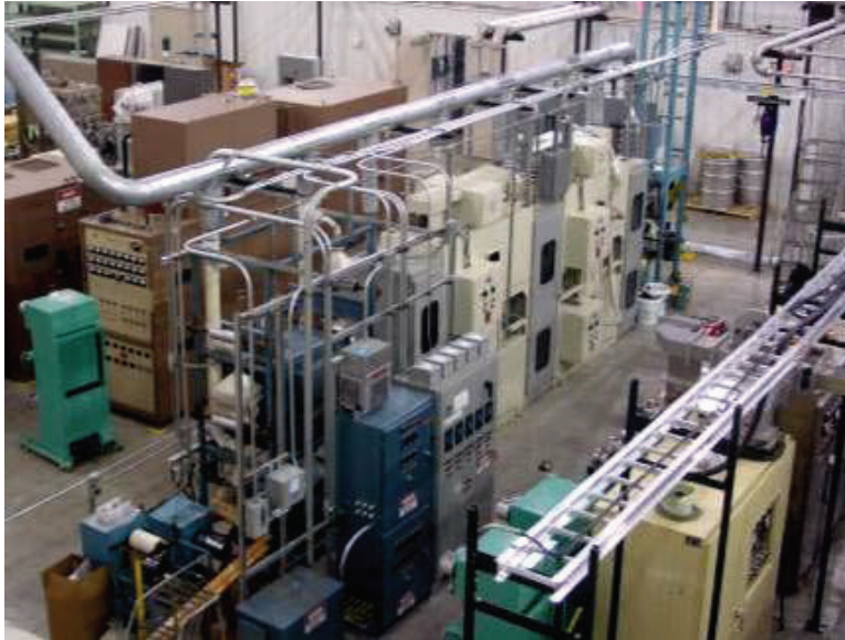
Carbon Fiber Technology Facility pilot line being upgraded for automated operation and production of high-strength CF.
