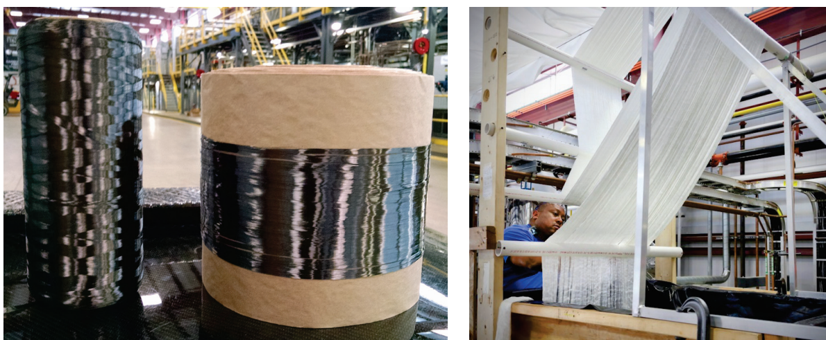
(Left) Typical spools of (a) 24 K industrial-grade carbon fiber and (b) 610 K rolls of textile-based carbon fiber. (Right) Carbon fiber produced at CFTF using a textile acrylic fiber.
