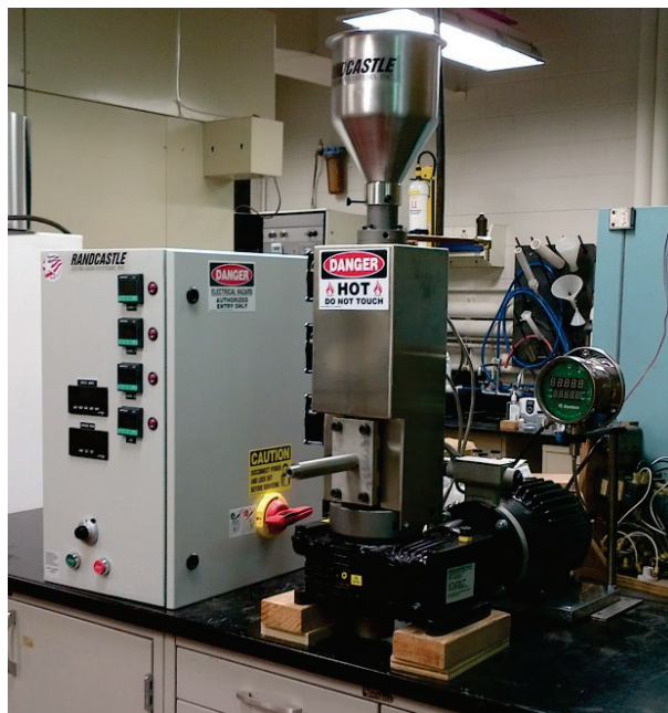
Randcastle 5/8 in. screw extruder in the processing lab at Virginia Tech.
