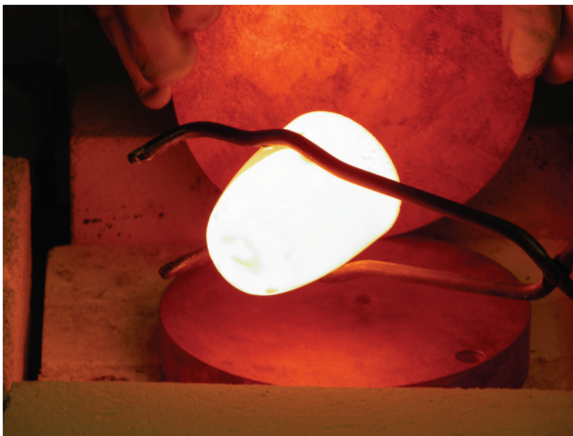
ORNL glass cathode materials are usually formed by splat quenching, in which molten glass is cooled rapidly between two copper plates.
