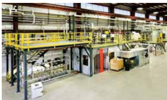
In-line precursor and carbon fiber production equipment.
