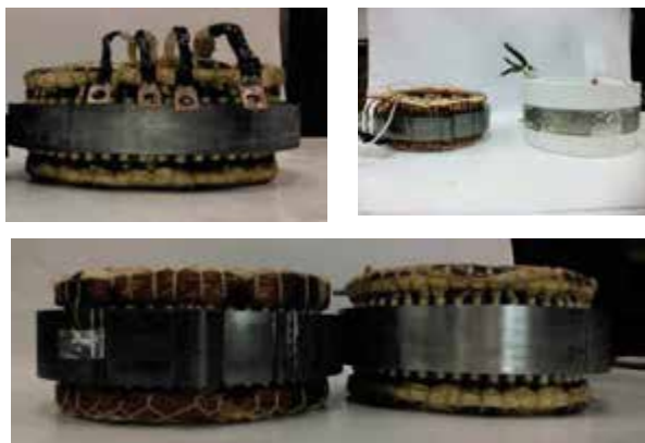
Stators fabricated for thermal and performance comparisons.
