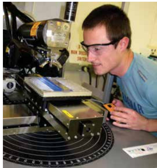
UTRC's Mike Humbert examines the alignment of a series of titanium alloy samples before XRD data collection at ORNL's HTML.
