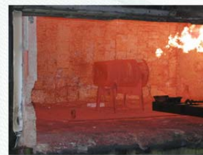
Package free drop and thermal tests per 10 CFR 71
