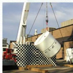
Package free drop and thermal tests per 10 CFR 71
