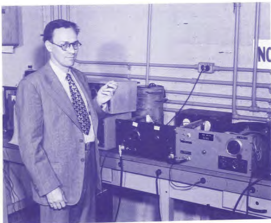
P. R. Bell checks the scintillation spectrometer he developed. In March 1949, this development was lauded as an "advancement of great significance in the field of radioactivity detection."
