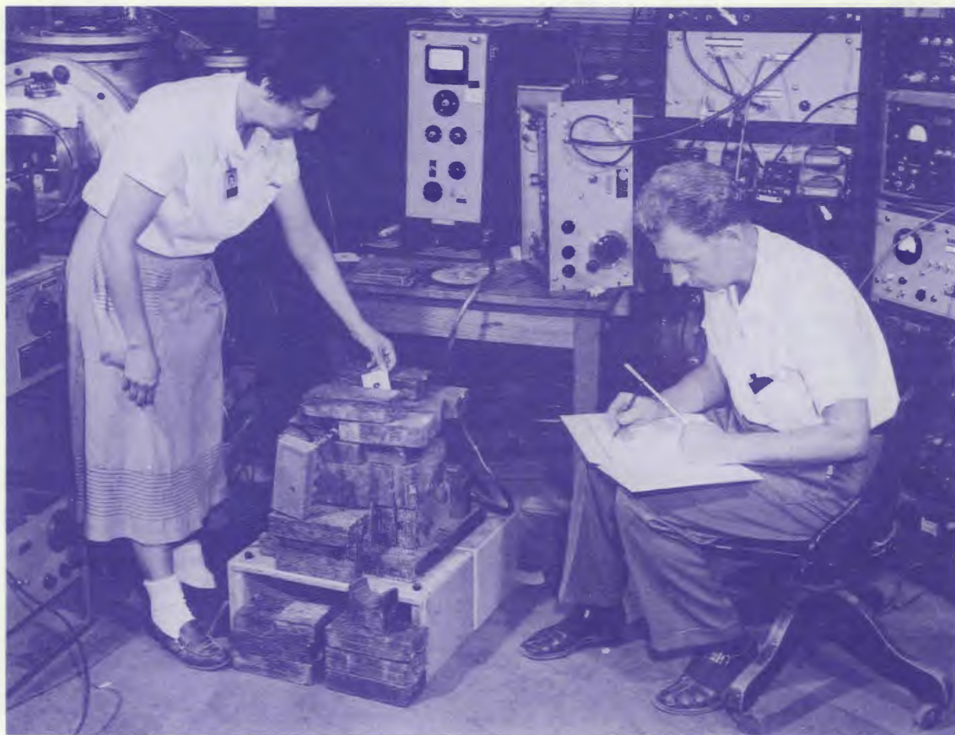
Frances Pleasonton and Art Snell check the performance of the coincidence circuits used in their 1951 experiment for detecting the radioactive decay of the neutron. The coincidence counters were temporarily built into a pile of lead bricks into which Miss Pleasonton inserts a radioactive source used for testing.
