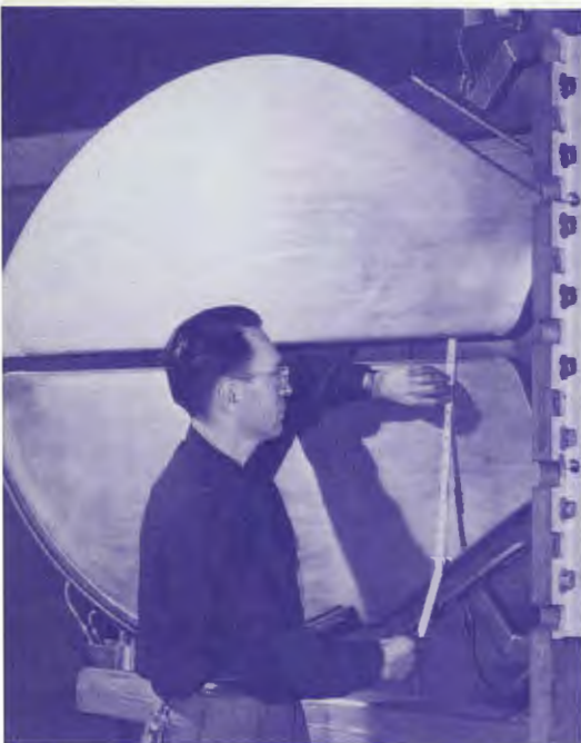
H. C. Hoy measures the distance between the big Ds of the 63-in cyclotron, shiny and new in 1952.
