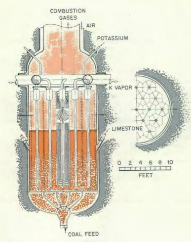
In this fluidized-bed combustion chamber and potassium boiler, the liquid potassium circulates in vertical, 1-in. tubes, which connect at the top with vapor separators, from which the vapor heads horizontally toward the turbine. Condensed potassium and the separated-out liquid potassium are sent to the bottom of the hot bed of coal and limestone via the 4-in. downcomer tubes.
