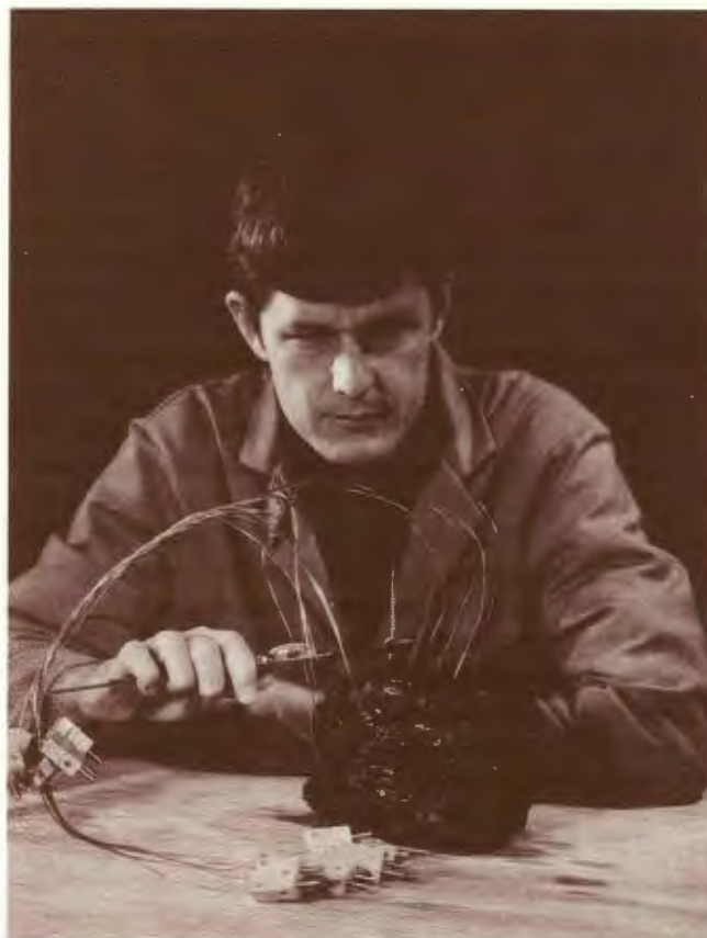
Richard Forrester of the Chemical Technology Division examines a lump of coal for heat transfer properties, information that will assist the country's research into in situ coal gasification processes.
