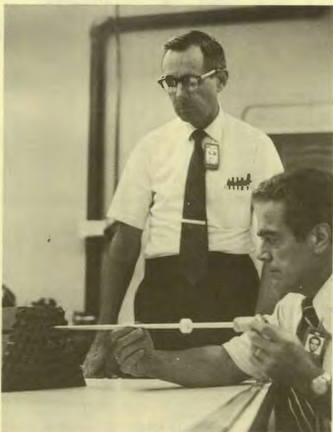
Pete Patriarca inserts a probe for introducing gamma-ray-producing isotopic pill into a tube to test for possible flaws in the joint between the tube and tubesheet. Bob McClung inspects this small section of tubesheet, a prototype of the intermediate heat exchanger of the CRBRP.
