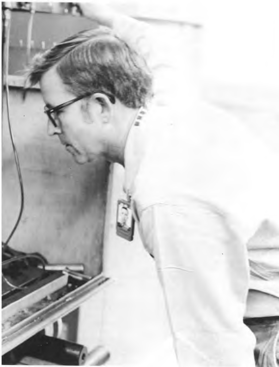
Claude Bengé, craftsman in Building 2525 (the "green door" shop), watches while the electrical discharge machine (EDM) performs the specialized sectioning of the postflight sample of copper-silver braze that was tagged with the silver-110 isotope.
