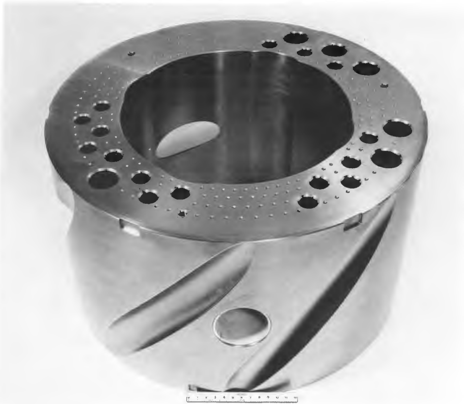
The neutron reflector which surrounds the fuel assembly and control cylinders is one of the largest beryllium components ever machined.
