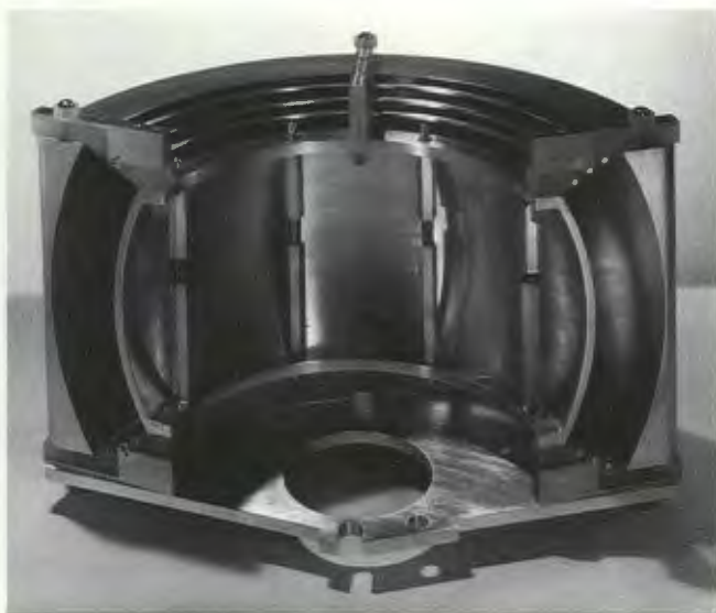
The double-focusing electrostatic plates, designed by Carlson and built by Frank Ward, Plant and Equipment Division, in 1968. The plates have the same basic design as those on the left but are machined for higher resolution.
