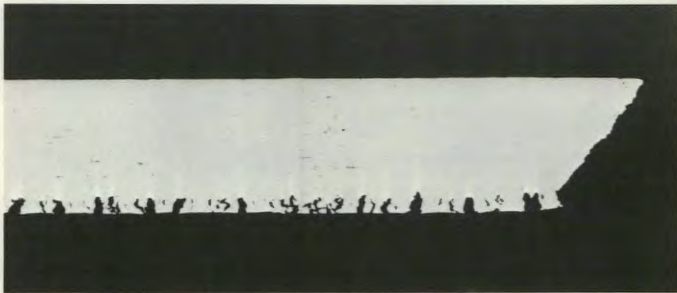
Fig. 5. Surface cracking in Hastelloy N exposed to MSRE fuel salt for 23,000 hours. The cracks penetrate to a maximum depth of 7 mils.
