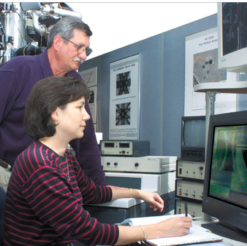
During DOE programs to advance industrial ceramic matrix composites, ORNL materials scientist Karren More (foreground, with former ORNL colleague Larry Walker) used transmission electron microscopy and other techniques to pinpoint causes of failure in stress- or field-tested materials made by companies. Image credit: ORNL
