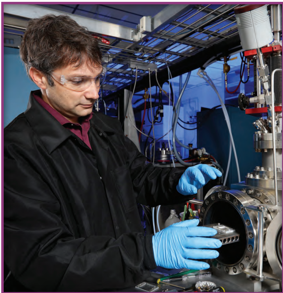
ORNL experimental chemist Gabriel Veith loads a deposition chamber to prepare battery samples. Image credit: Jason Richards
