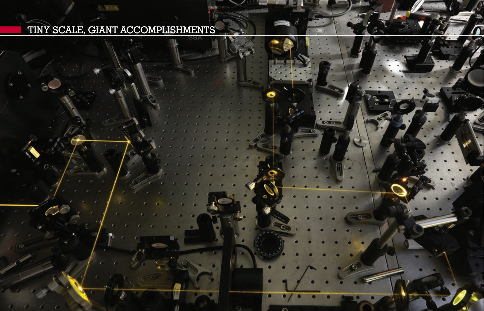
The laser-based ultrafast spectroscopy equipment at ORNL's Center for Nanophase Materials Sciences allows researchers to study phenomena in materials that happen on a timescale of a millionth billionth of a second. Image credit: Jason Richards, ORNL
