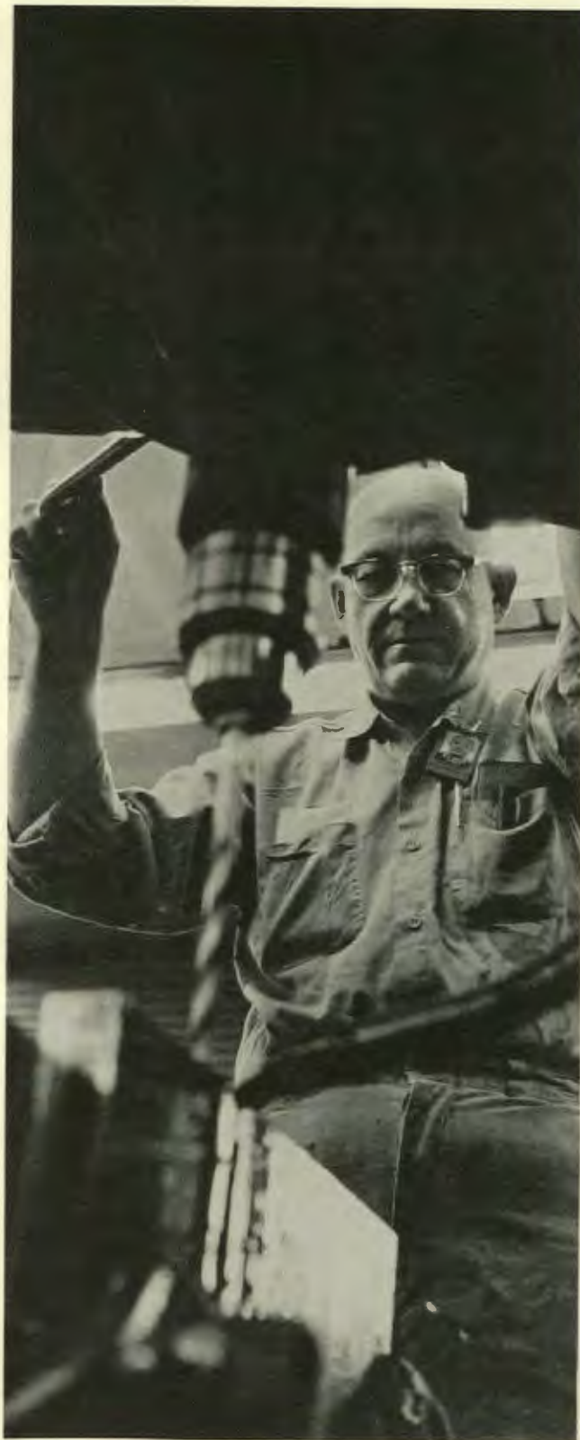
To drill a deep hole in a large metal part, W. A. Baker employs a long bit in the radial drill press.
