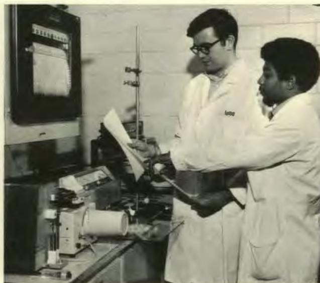
Ray Fenwick and Ron Sheehy operate a scintillation spectrometer in Prof. Roy Curtiss's laboratory.
