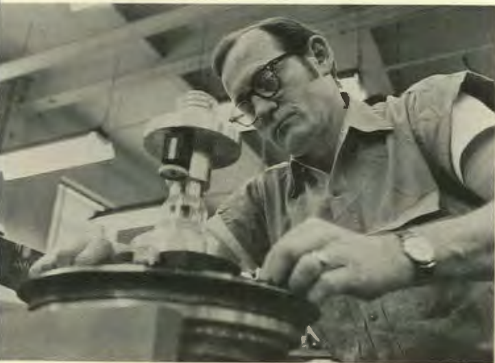
To position a crystal in a cryostat the proper equipment is a goniometer such as the one R. E. Hopper assembles here in the shop at 3025.
