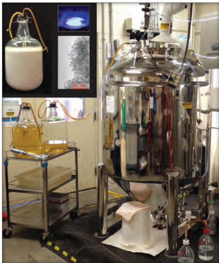
Using this 250-gallon reactor, ORNL researchers produced three-fourths of a pound of zinc sulfide quantum dots, shown in the inset. Image credit: ORNL
