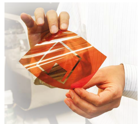
ORNL researchers are experimenting with additive roll-to-roll manufacturing techniques to develop low-cost wireless sensors. ORNL's Pooran Joshi shows how the process enables electronics components to be printed on flexible plastic substrates. Image credit: Jason Richards, ORNL
