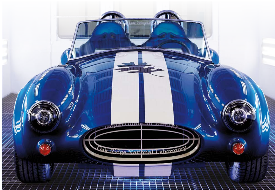
This replica Shelby Cobra was printed at DOE's Manufacturing Demonstration Facility at ORNL using the Big Area Additive Manufacturing machine. BAAM can manufacture strong, lightweight composite parts larger than a cubic meter. This Cobra comes in at about 1,400 pounds and contains 500 pounds of printed parts made of 20 percent carbon fiber. Image credit: Genevieve Martin, ORNL. For more information: http://go.usa.gov/3W9SA
