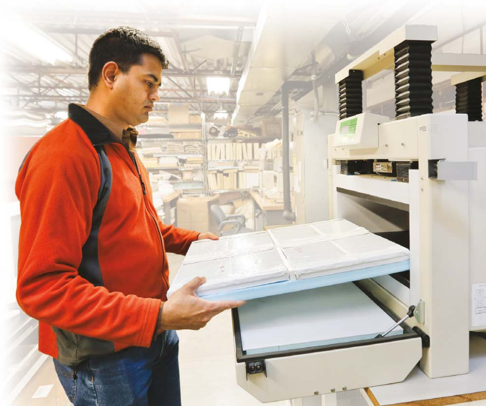
ORNL researcher Kaushik Biswas analyzes the thermal performance of a 2-by-2 foot composite panel covered with smaller modified atmosphere insulation panels separated by foam insulation. Image credit: Jason Richards, ORNL
