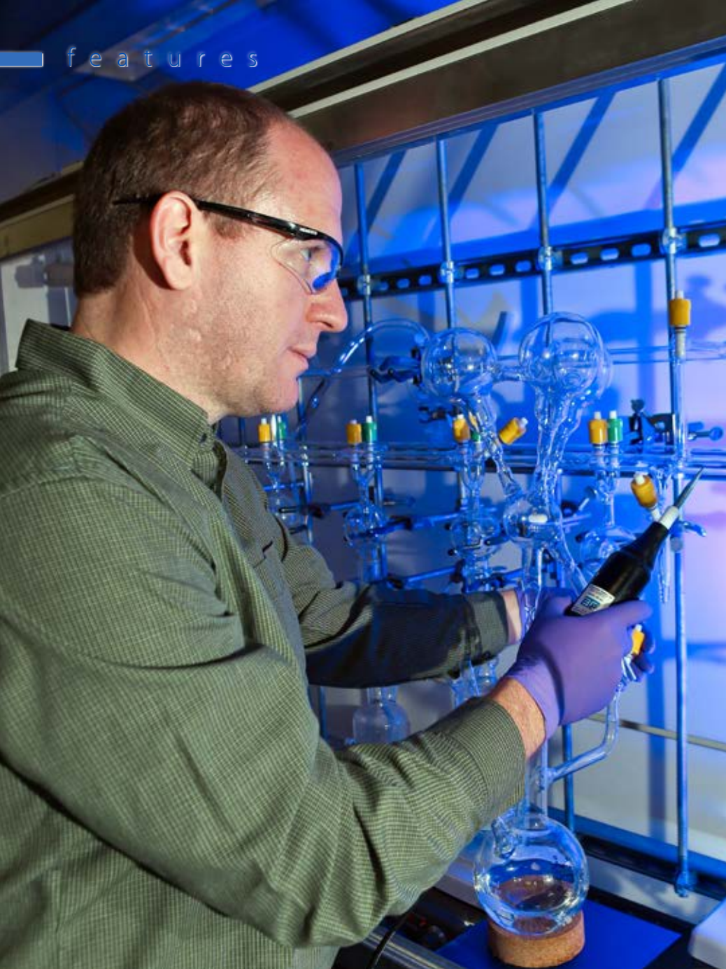
Materials scientist Jamie Messman uses a Tesla coil to test the vacuum of a polymer synthesis apparatus. (Photo: Jason Richards)
