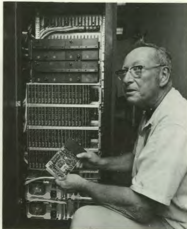
Arnold Kenerly, instrument technician who performs most of the maintenance on the system, holds one of the operational amplifiers in back of the analog console.
