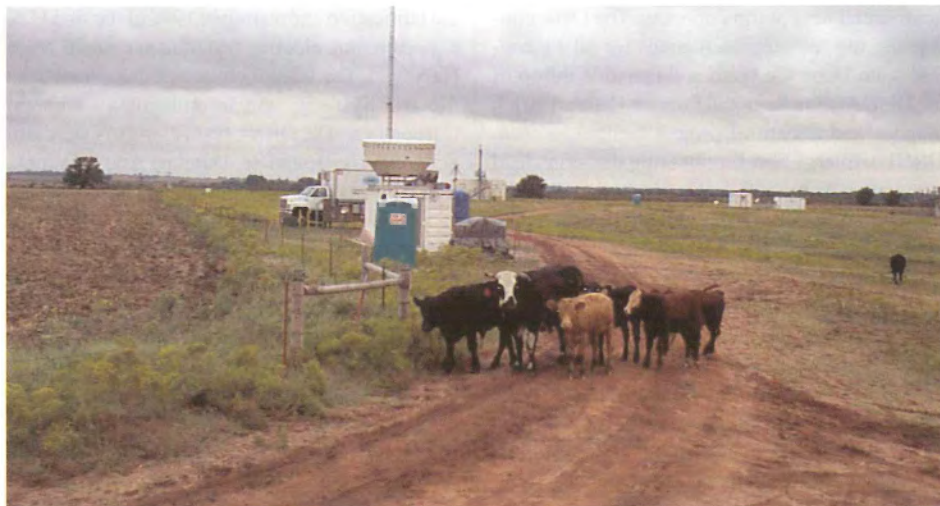
This ARM millimeter cloud radar instrument in Oklahoma cattle country enables scientists to determine whether a cloud contains mostly ice crystals or liquid water. Such measurements help scientists predict the degree to which the cloud reflects, absorbs, or transmits sunlight.
