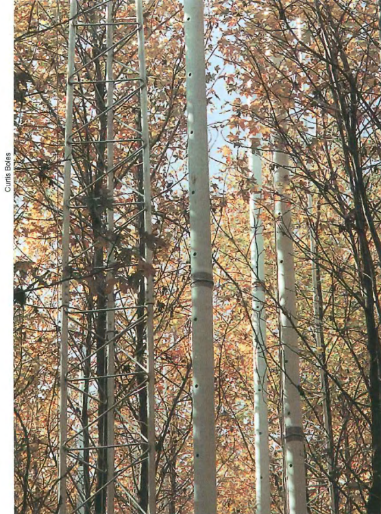
Standing tall in a small sweetgum plantation are a tower and vent pipes that provide the trees with additional amounts of carbon dioxide. This hardware is part of ORNL's novel free-air \text{CO}_2 enrichment system. During the first year of exposure to the increased \text{CO}_2 concentrations, the trees grew faster and conserved water.
