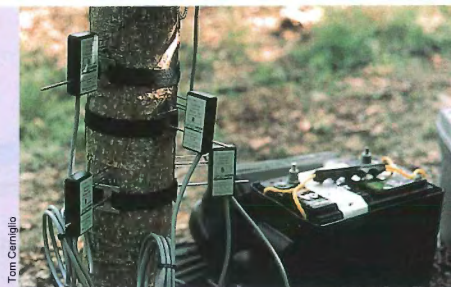
This series of heat-pulse probes inserted at various depths in a cottonwood tree provide measurements to help ORNL scientists estimate whole-tree water use in an experiment examining the interactions between genetics and environment in determining plant growth and productivity. This research is part of a CRADA project with Union Camp Corporation.
