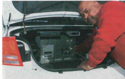
Here, Ron Harris connects the device controlling the lane tracker system with a computer.
