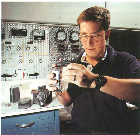
James Klett demonstrates the rapid melting of an ice cube applied to a carbon foam sample held in his hand. The sample transfers heat from his hand rapidly to the ice cube, causing the cube to melt quickly and his hand to feel suddenly cold. Such carbon foam could prove useful for making car radiators.
