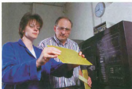
April McMillan and Felix Paulauskas examine the result of using microwave energy to bond two glass-fiber-reinforced composite parts.
