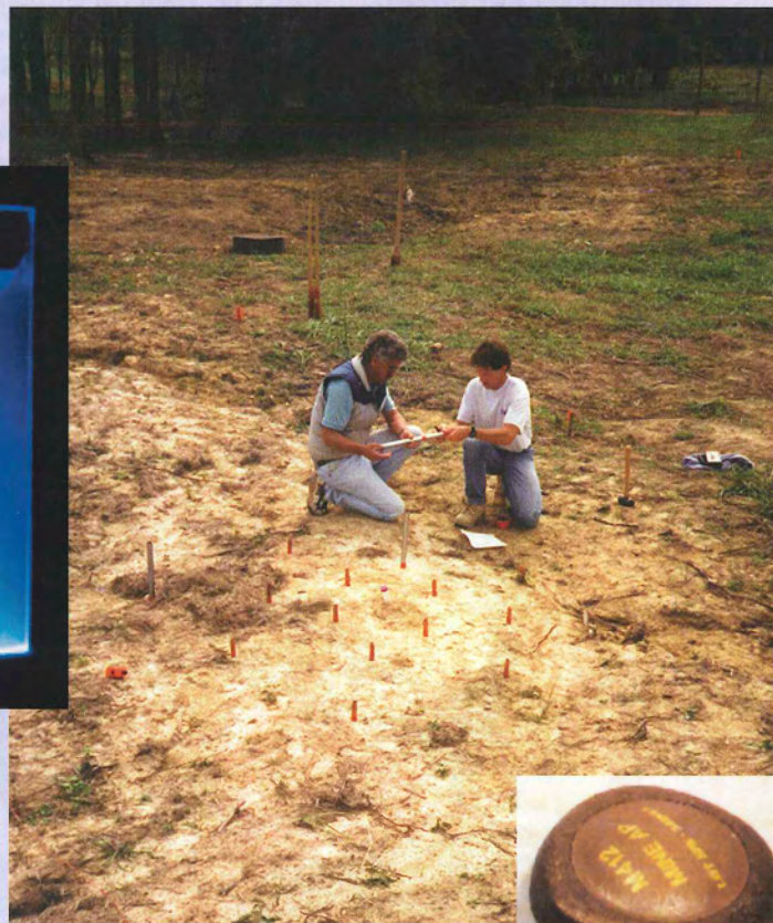
Mike Maston (left) and Billy Schaefer examine an area around a land mine, taking soil samples from a site that was identified as a mine using the ORNL Microbial Mine Detection System. The insets show a tube of the microorganism as it fluoresces and a typical antipersonnel mine.
