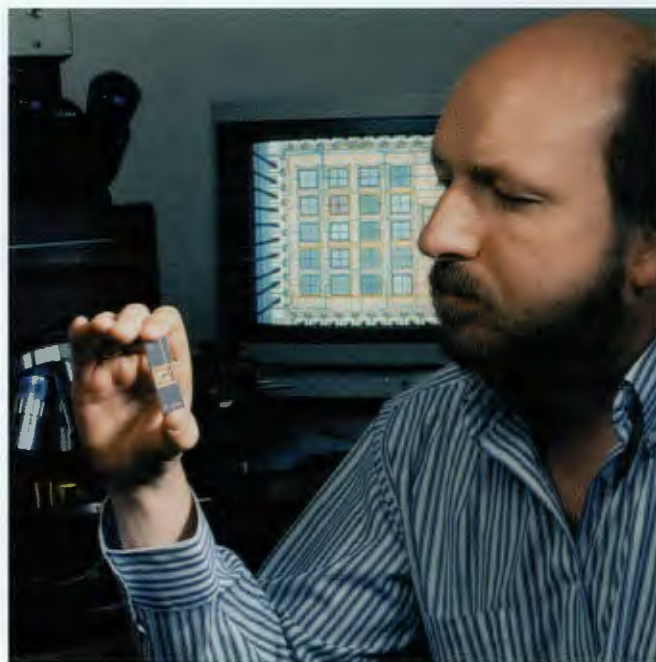
Mike Simpson shows the bioluminescent bioreporter chip, dubbed the critters on a chip. Genetically engineered bacteria on the chip emit blue-green light when they encounter a pollutant they like to eat. The light is detected by the chip electronics, and the resulting electrical signal reveals the identity and concentration of the pollutant.
