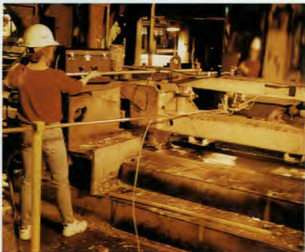
ORNL engineer Ruth Ann Abston adjusts the phosphor deposition device in front of the galvanneal sheet.
