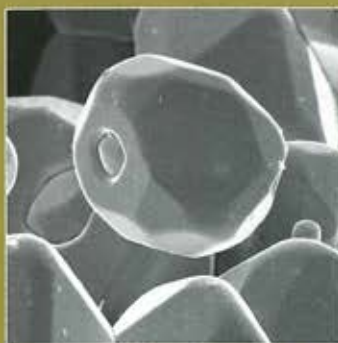
These micrographs show the microstructural results of reacting at high temperatures (up to 700°C) and high pressures (1050 bars) various samples of fine-grained magnetite with a solution of salt (sodium chloride) and water containing different oxygen isotope ( ^{18}\text{O} and ^{16}\text{O} ) compositions. The research was performed by David Cole using funds from the Geosciences Research Program of DOE's Office of Basic Energy Sciences.
