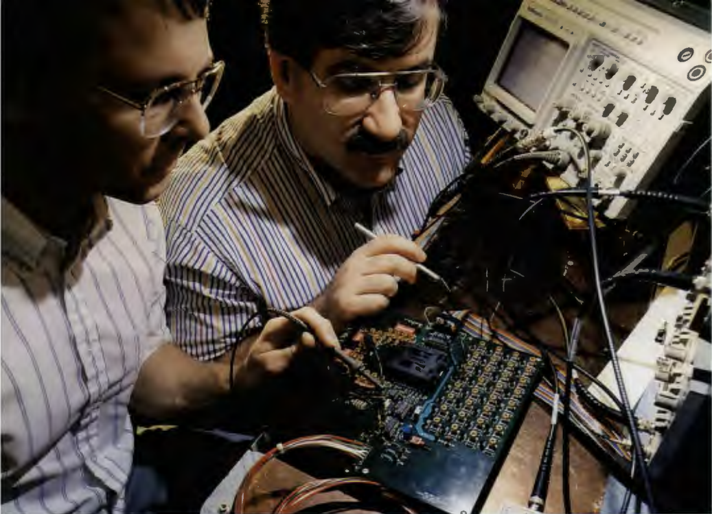
Alan Wintenberg (left) and Glenn Young check a fixture for testing ORNL-designed integrated-circuit electronics for a silicon detector being developed for the quark-gluon plasma experiment at Brookhaven National Laboratory's Relativistic Heavy Ion Collider. The experiment could help scientists better understand the actions of subatomic particles in the universe at the start of the Big Bang.
