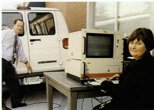
Tim Hickerson and Vivian Baylor operate the heartbeat detector in an attempt to detect the presence of a human hidden in the truck.
