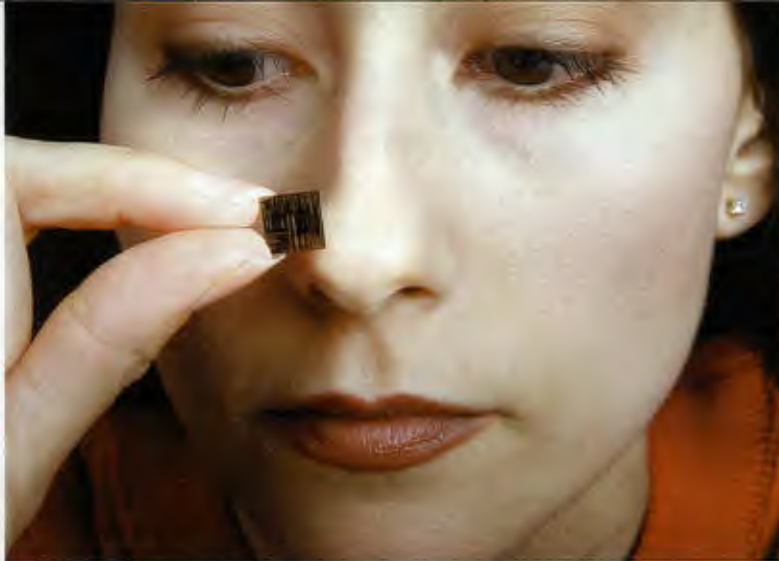
Kim Young examines the "nose on a chip," which uses cantilevers coated with different chemicals to detect multiple gases.
