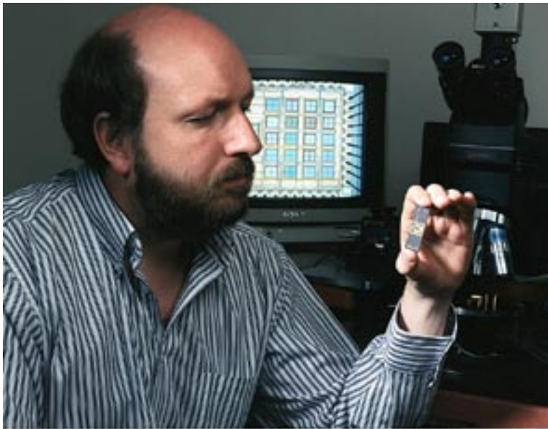
Mike Simpson examines the bioluminescent bioreporter chip (magnified on the monitor in the background). Genetically engineered bacteria on the chip emit blue-green light when the pollutant is detected. The chip detects this light. Photograph by Tom Cerniglio.
