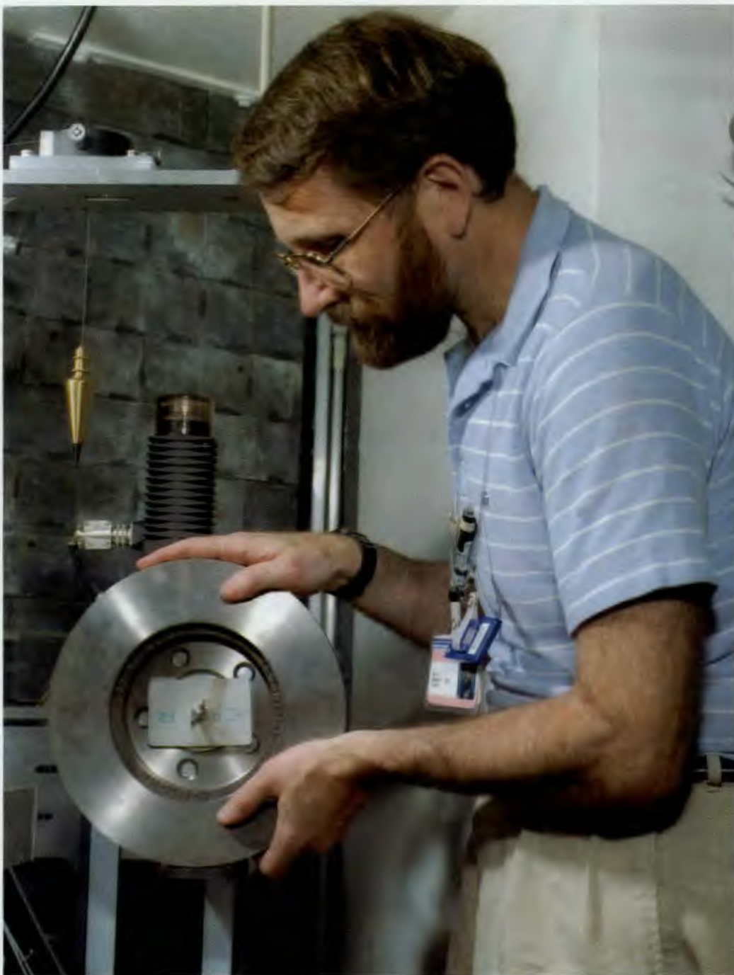
Bill Donlan, a Ford Motor Company researcher, prepares to use neutrons from ORNL's High Flux Isotope Reactor to map residual stresses in automobile brake discs. Photograph by J.W. Nave.
