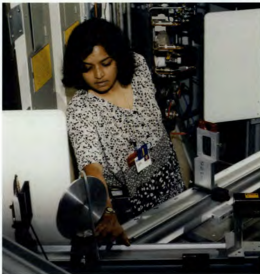
Mona Yethiraj, an ORNL scientist, checks a small-angle neutron scattering spectrometer that will be operated remotely for neutron science experiments at ORNL's High Flux Isotope Reactor.
