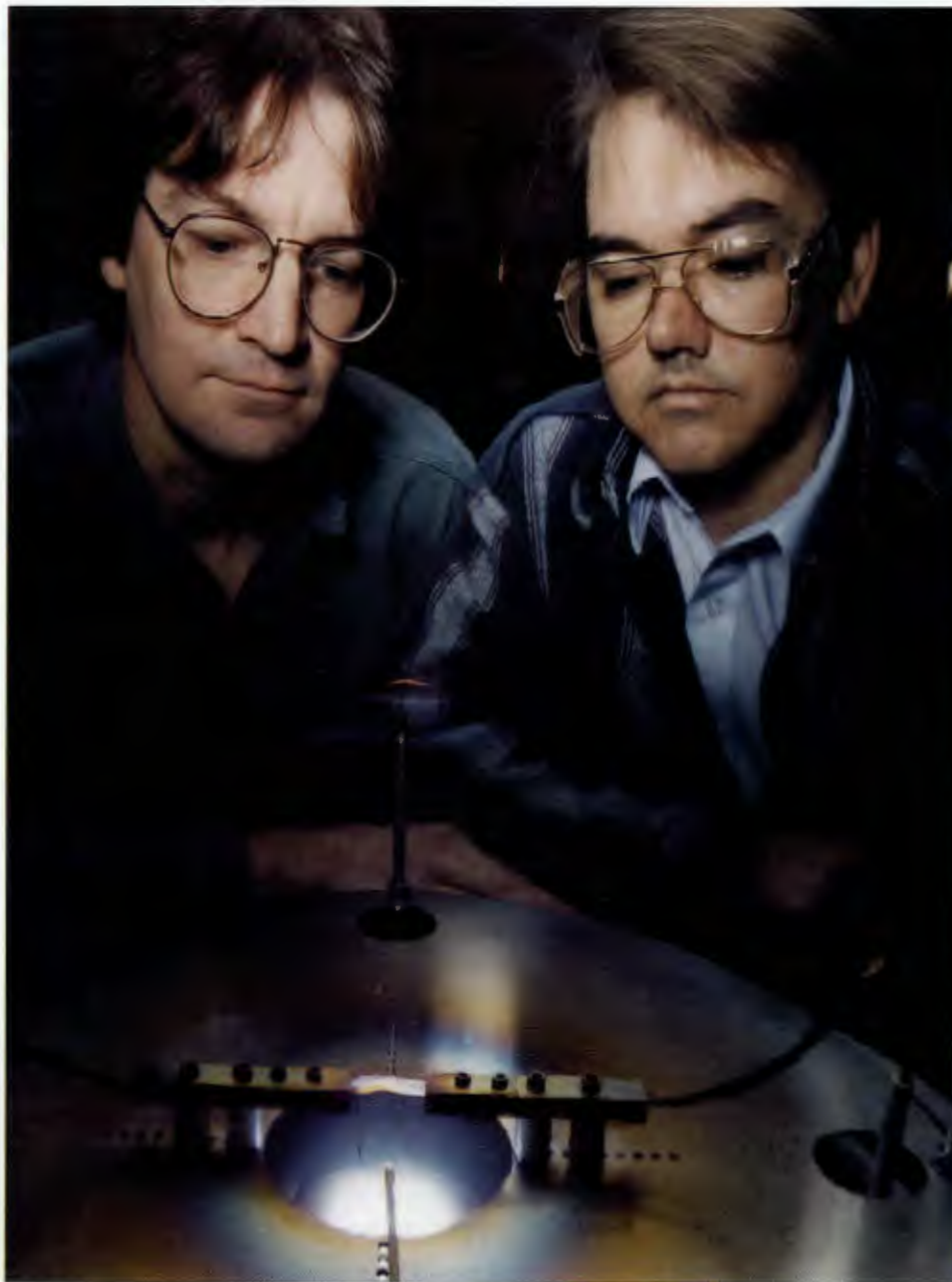
Fred List (left) and Patrick Martin observe sputtering of cerium oxide on textured nickel, the substrate for high-temperature wire capable of carrying large amounts of current. Photograph by Tom Cerniglio.
