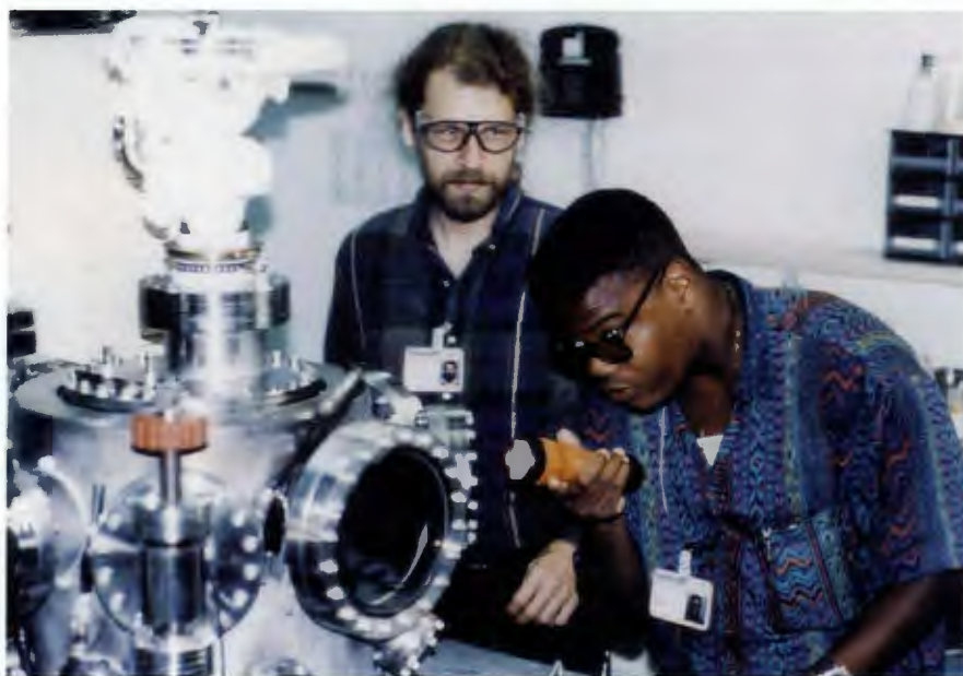
Eric Williams (left) and Melvin Spurlock, graduate students at Alabama A&M University, help perform materials research at ORNL’s Surface Modification and Characterization Research Center. Here, Spurlock examines a sample in a target chamber, which will be implanted by ions from an accelerator.
