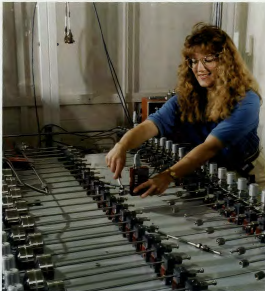
At the Metrology Research and Development Laboratories facility, mechanical engineer Ruth Anne Abston prepares a mass flow controller for testing by ORNL's prize-winning gravimetric calibrator, which measures gas flow rates. Photograph by Curtis Boles.
