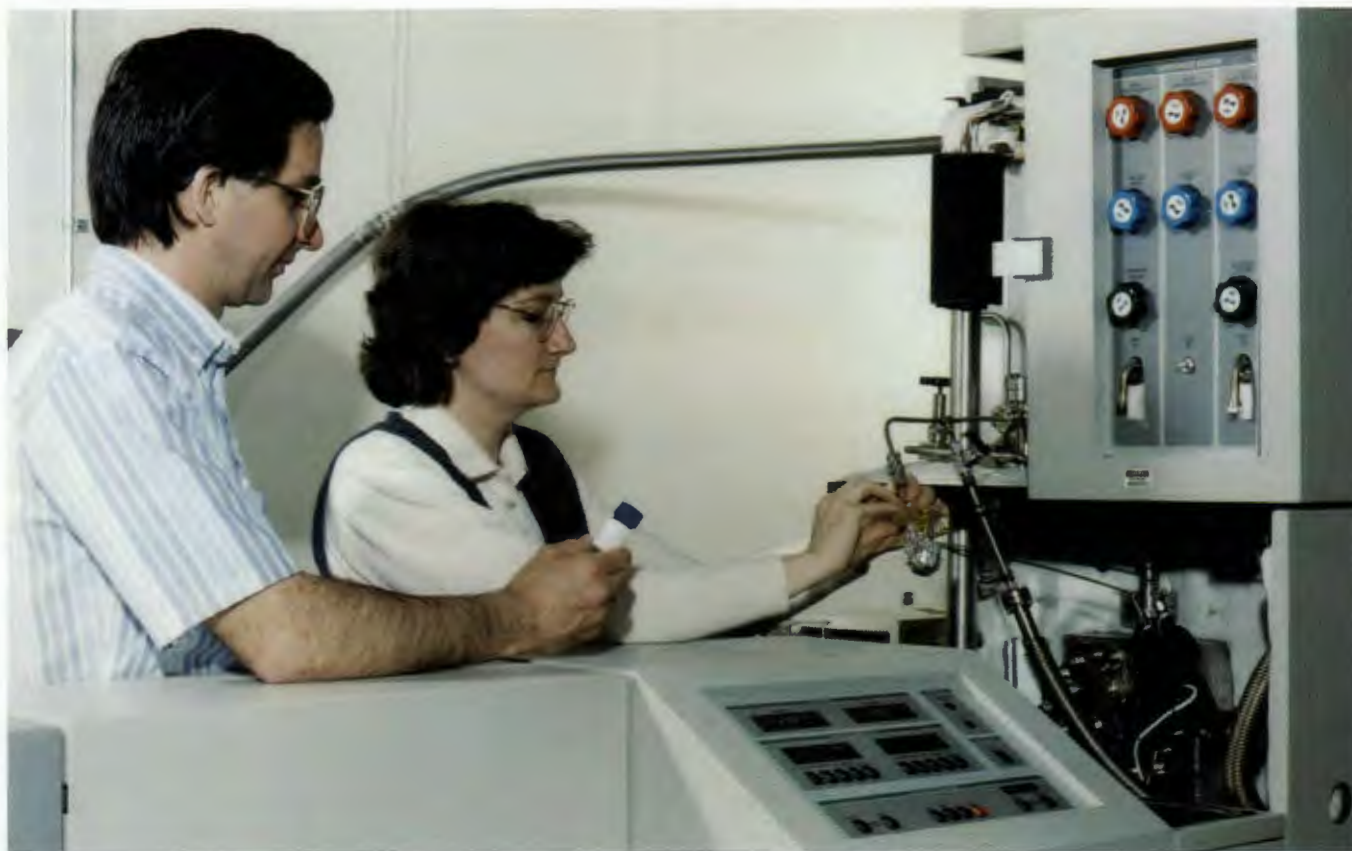
Bob Hettich and Michelle Buchanan prepare to analyze modified DNA oligomers on ORNL's 3-tesla Fourier transform ion cyclotron resonance (FTICR) mass spectrometer. A 7-tesla instrument that was to be installed in mid-1996 will substantially enhance achievable mass range and mass resolution for analysis of biomolecules. Photograph by Curtis Boles.
