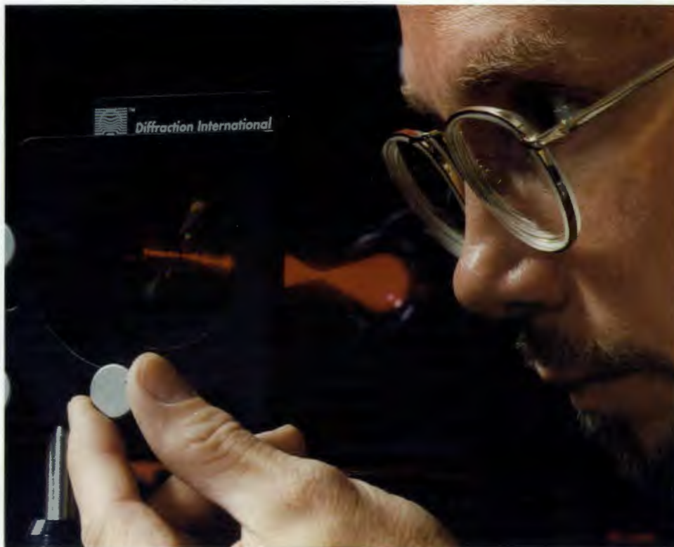
Curt Maxey aligns the CGH Null Adapter using a specialized computer-generated hologram. In conjunction with custom CGH null lenses, the product enables aspheric optics to be tested with conventional interferometers to ensure they have the right shape. Photograph by Lynn Freeny.
