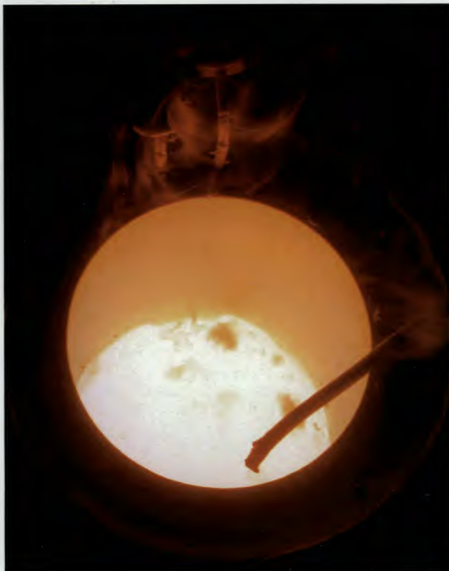
ORNL researchers developed the Exo-Melt furnace concept for efficiently and safely melting and casting alloys of nickel and iron aluminide. Photograph by J.W. Nave. Computer photo enhanced by Mark Robbins.
