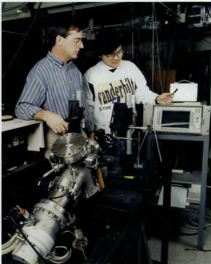
Steve Allman (left) and Kai Tang are part of the team that developed the laser mass spectrometer for detection of genetic defects that can lead to cystic fibrosis.
