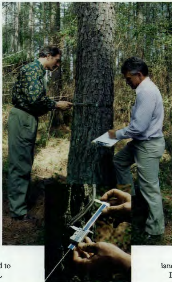
Sandy McLaughlin (left) and Darrell Downing precisely measure the growth of loblolly pine trees in a forest exposed to high ozone levels and hot, dry conditions. Inset: Growth of each tree was monitored by a dendrometer, a metal band positioned around the trunk that precisely measures fluctuations in its expansion rate. Photograph by Tom Cerniglio.
