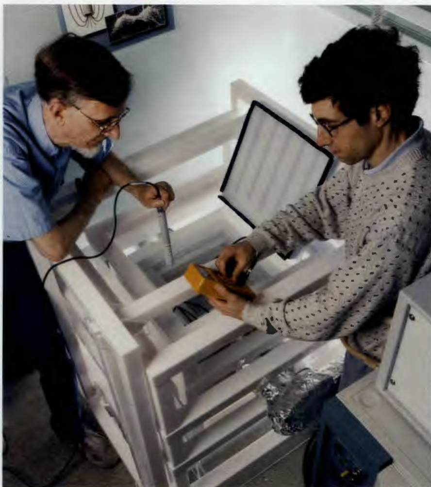
Guy Griffin (left) and Paul Gailey use a fluxgate magnetometer to perform a calibration check of ORNL's magnetic field exposure system, which exposes biological cell cultures to precise magnetic fields in an environment in which temperature, humidity, and carbon dioxide are controlled. Cell cultures are placed in two chambers, but the control electronics turn on exposure fields in only one (and the researchers don't know which one, ensuring that no inadvertent bias enters the experiments). Photograph by Tom Cerniglio.
