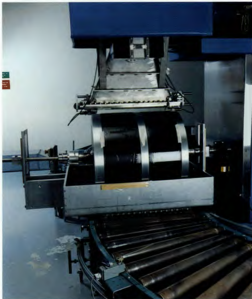
ORNL conducts experiments in producing polymer-composite parts using a continuously operated electron-beam system in western Canada. The electron beam scan horn at top center directs and controls distribution of electrons to composite test parts.
