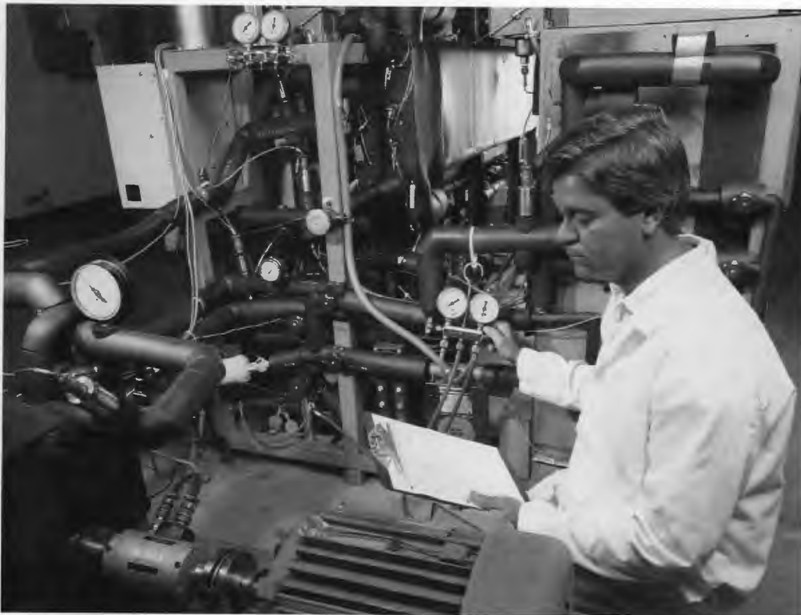
Ed Vineyard checks instrument readings during a test of chlorine-free refrigerant mixtures and alternatives to the coolant HCFC-22.
