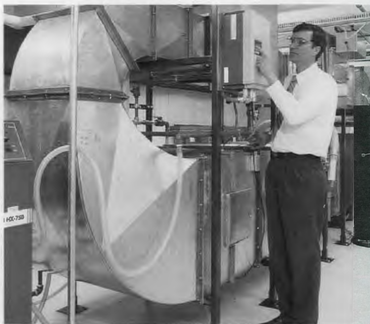
Bill Miller inspects a facility for testing heat exchanger designs for advanced heat pump systems.
