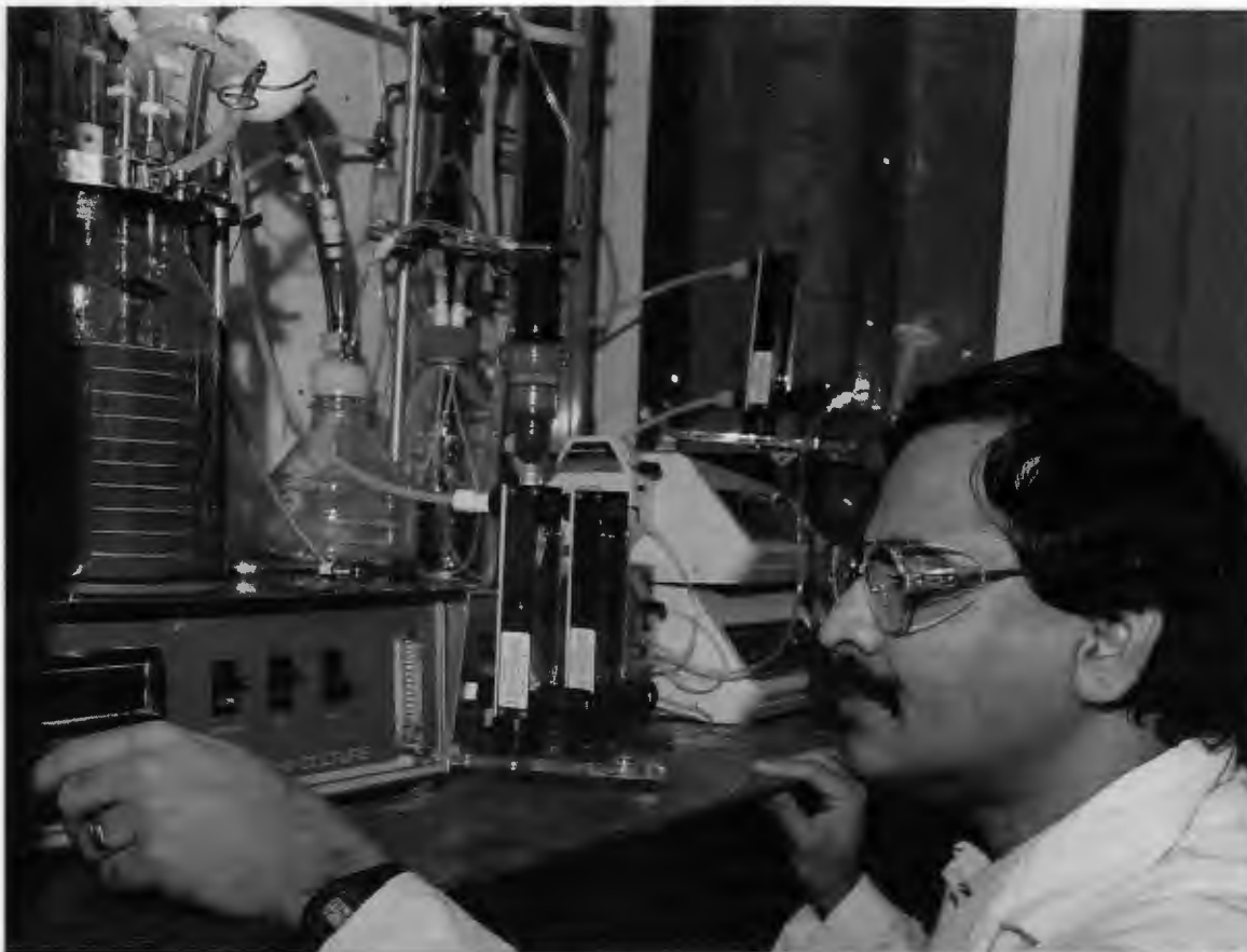
P. T. Selvaraj, a postdoctoral scientist with the Bioprocessing Research and Development Center at ORNL, adjusts controls on a bioreactor. The glass vessel contains bacteria in beads suspended in sewage media. Sulfur dioxide, a coal power plant pollutant, is passed through the bioreactor, and the bacteria convert the pollutant to hydrogen sulfide for subsequent conversion to sulfur, a useful product.
