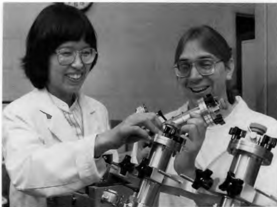
Liyuan Liang and John Goodlaxson adjust the zero-headspace extractors for studies of the effectiveness of iron and palladium in removing chlorine from organic compounds found in contaminated groundwater.
