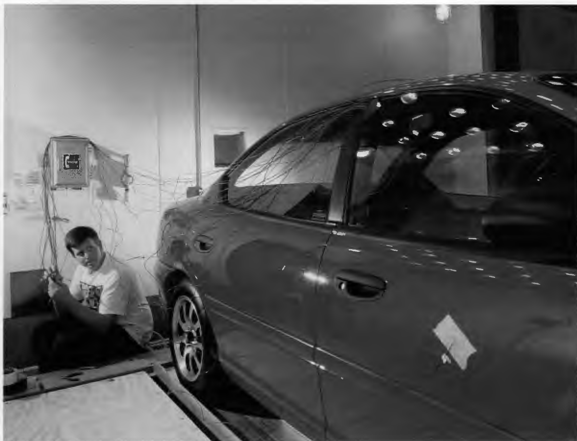
Mark Valk, a University of Tennessee senior mechanical engineering student, prepares a 1995 Chrysler Neon for a test in the Large Scale Climate Simulator at ORNL's Buildings Technology Center. This hybrid electric vehicle placed first in its category in the 1995 Hybrid Electric Vehicle Challenge held in June 1995 in Auburn Hills, Michigan.
