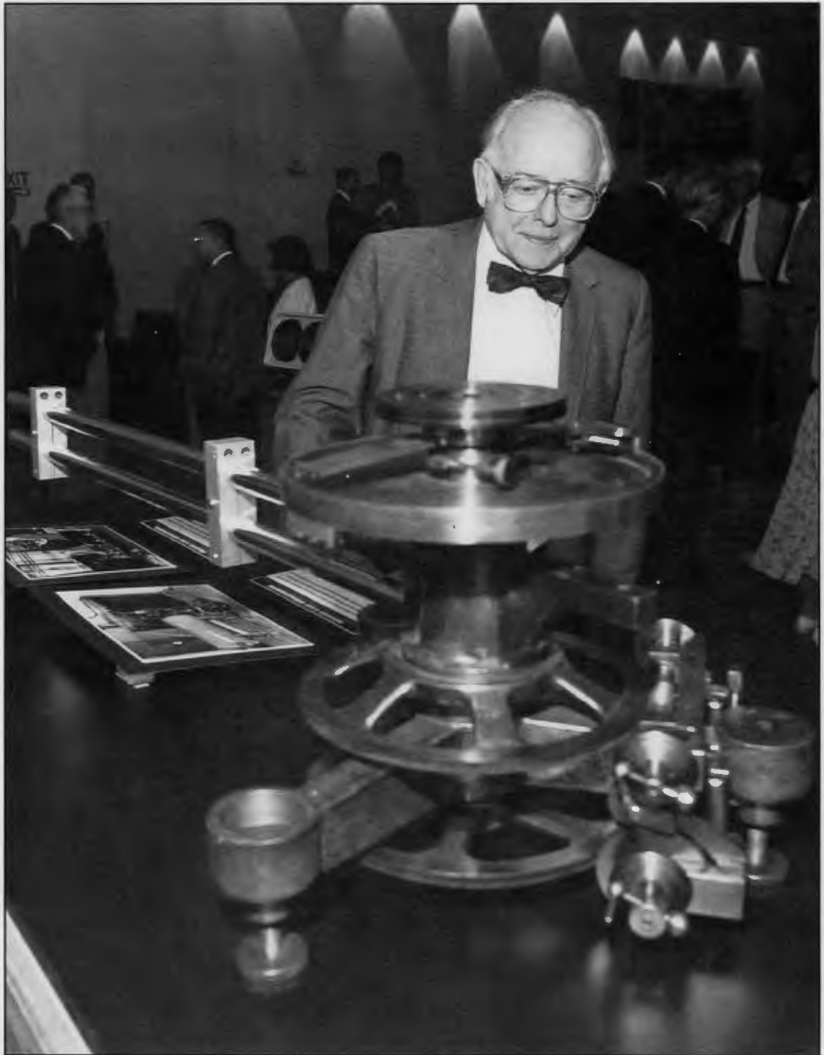
Nobel Laureate Clifford Shull examines the neutron diffractometer now on display at the American Museum of Science and Energy in Oak Ridge. Shull used this instrument for his neutron-scattering research at ORNL's Graphite Reactor.— Photograph by Kelley Scott Walli.
