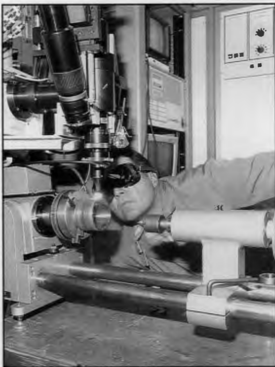
Russ Greeley, a materials joining technologist, watches two parts being welded together by a laser welder in the Materials Joining Center.
