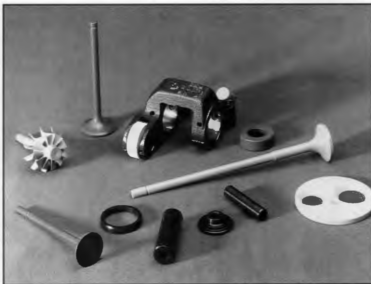
ORCMT staff are developing ceramic components for highly efficient gas turbine engines that will be operated at temperatures that would melt metal engine parts.
