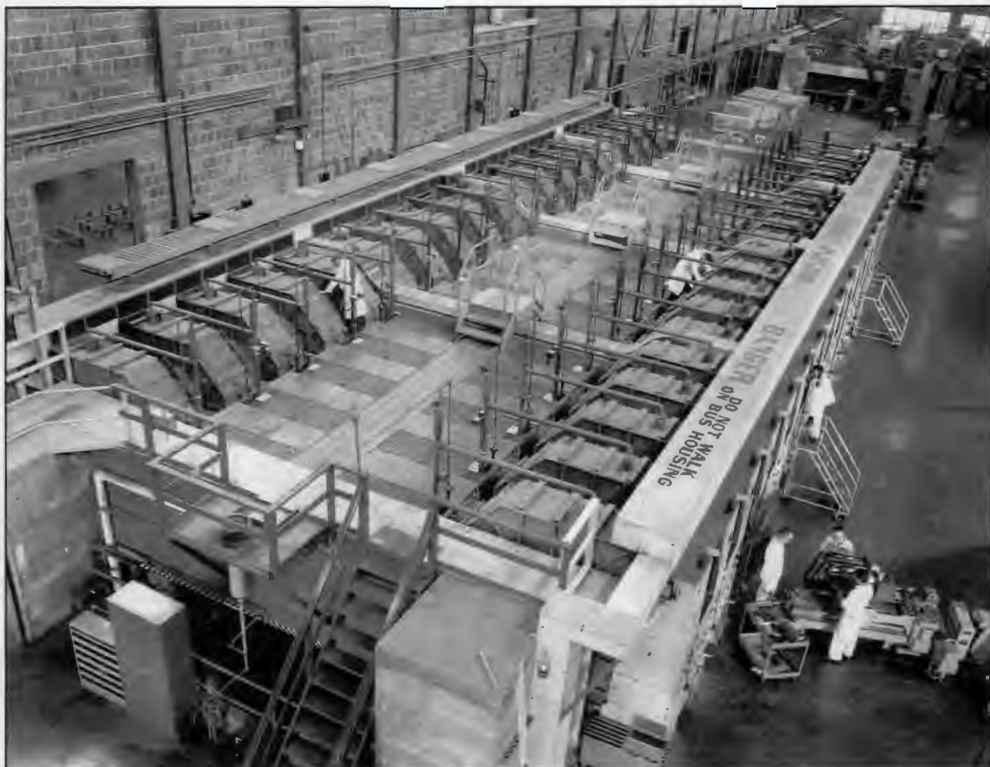
ORNL uses these calutrons at the Y-12 Plant to produce thallium-203, a stable isotope that is converted to radioisotope thallium-201 for heart scans. The calutrons were recently restarted after being idle for three years.
