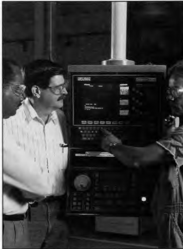
Mike Pelfrey (right) a machinist in the Skills Demonstration Center, explains the workings of a computer numerically-controlled three-axis milling machine to John Jordon and Don Garren.
