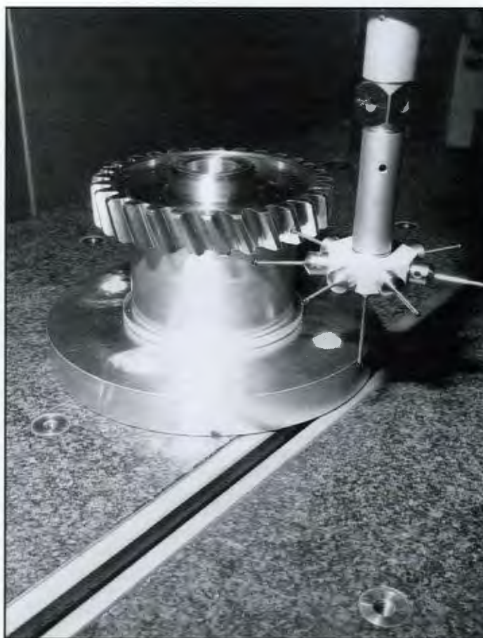
A coordinate measuring machine measures volume changes in heat-treated gears as part of the data gathering process for cooperative research conducted by DOE, several American automakers, the National Center for Manufacturing Sciences, and the Gear Research Institute.
