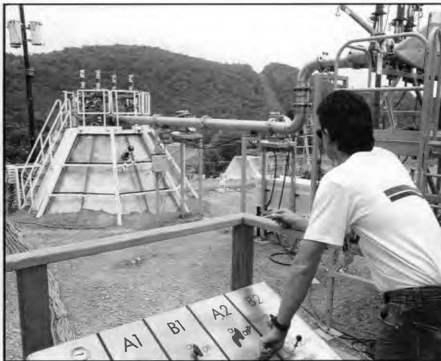
An in situ vitrification (ISV) test was performed at ORNL in 1991. In September 1995, ISV will be used to turn the soil in a radioactive waste pit into 600 tons of glass, immobilizing the contaminants.
