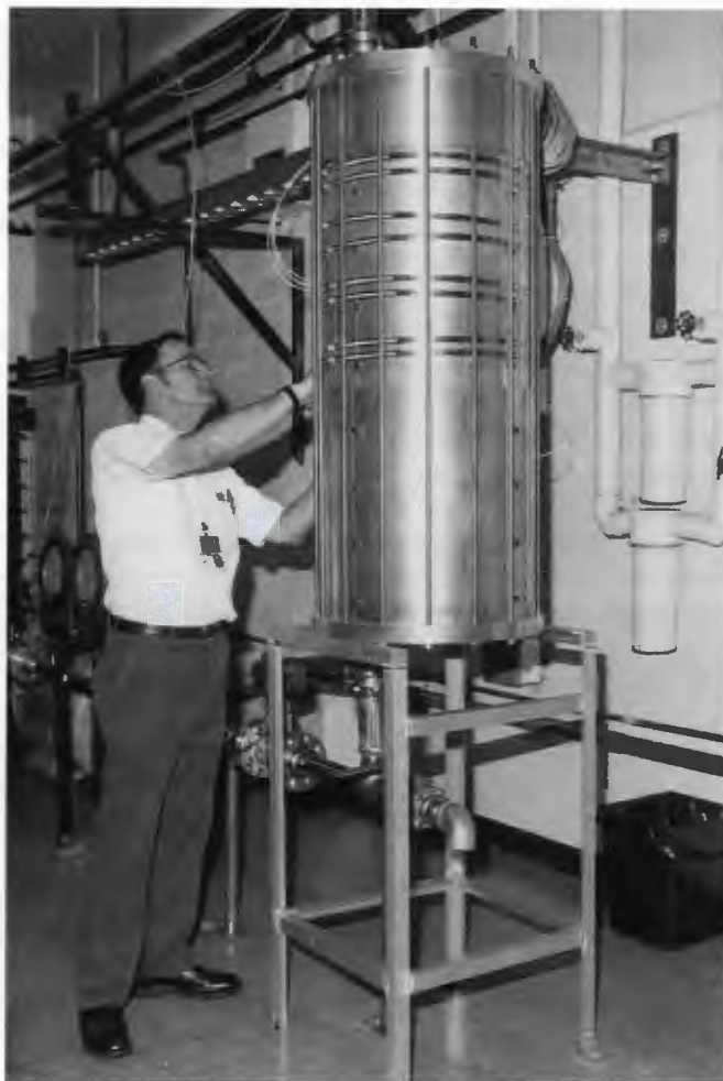
Frank Swinson adjusts the Plate Stability Test Facility used to evaluate fuel plate stability under ANS coolant flow conditions.
