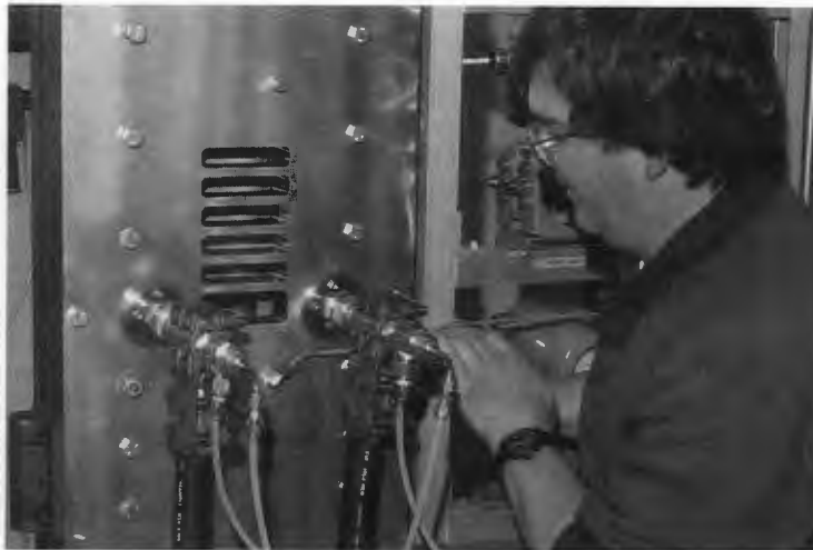
George Farguharson installs diagnostic heater connections on the Flow Blockage Test Facility. The facility provides temperature measurements using thermochromic liquid crystals and image processing in a mock fuel element. These continuous measurements are used to experimentally determine heat transfer downstream of a postulated flow blockage in an ANS-like core.
