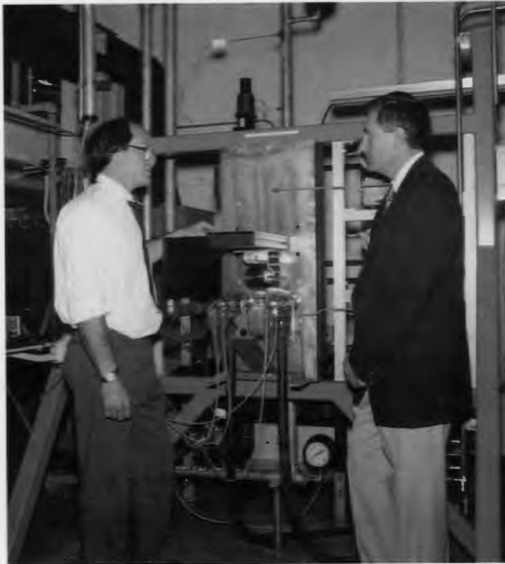
Dave Felde explains to Doug Selby some results from recent operation of the Flow Block Test Facility (shown here). It measures changes in the temperature of the fuel cladding as a result of a blockage in the coolant channel. The variations in temperature are recorded in color on film, and a camera transmits the color information to a computer, which analyzes and displays the results in color on the screen.
