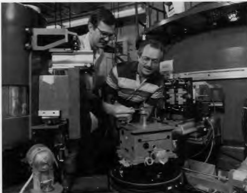
Jerel Zarestky (left), a user from DOE's Ames Laboratory, and Bob Nicklow, manager of ORNL's Neutron Scattering Research Facility, adjust the orientation of a cobalt manganese alloy using a triple-axis spectrometer. The machine measures the energy of neutrons scattered from the sample. Photograph by Bill Norris.
