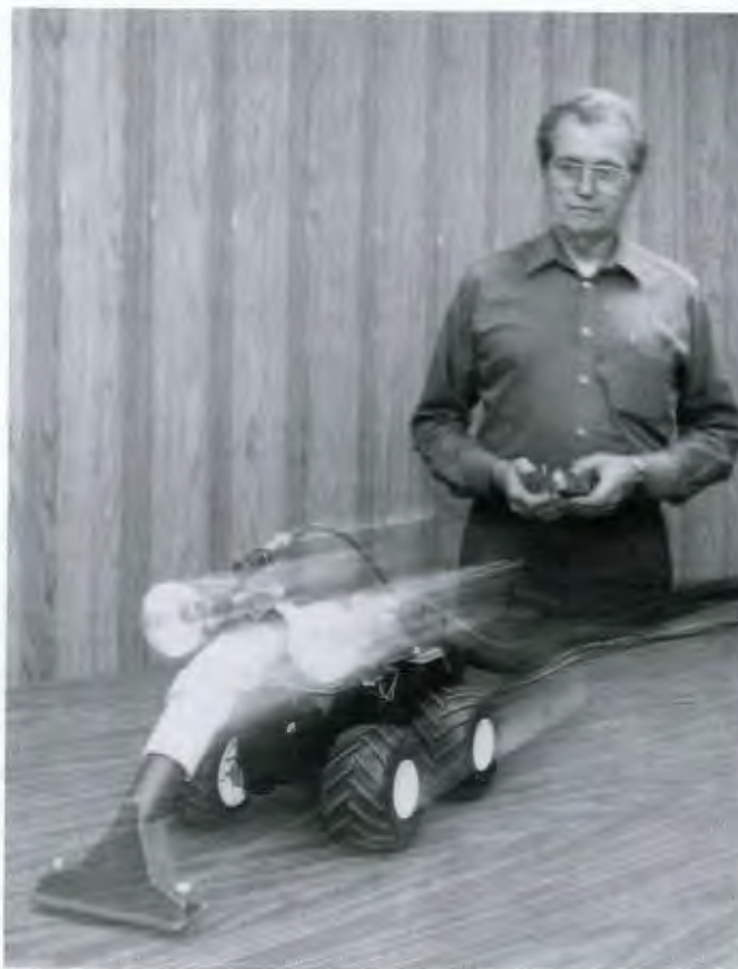
Don Box operates the remote-controlled vacuum cleaner used to remove trash from a tank at ORNL. Photo by Steve Eberhardt.
