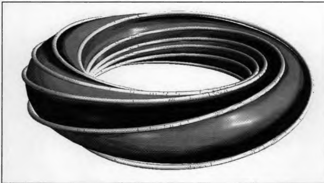
Scientific visualization of a toroidal surface inside a tokamak plasma with associated magnetic field lines. The shading of the toroidal surface is proportional to levels of turbulent fluctuation from a plasma instability in an experimental fusion reactor.
