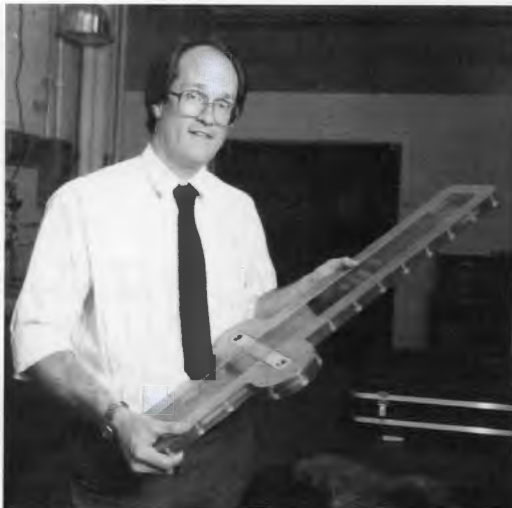
Dave Felde shows a coolant channel in which measurements are made on changes in the temperature of fuel cladding as a result of a channel blockage.
