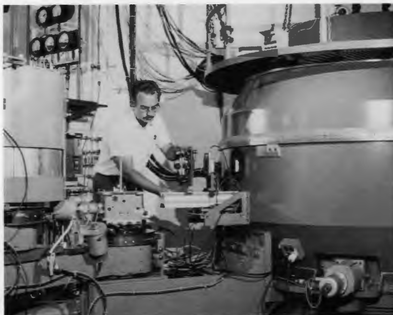
Bob Nicklow adjusts the beam aperture at the HB-3 triple-axis spectrometer, the type of instrument that will be available at the experimental workstations in the neutron beam room of the ANS.
