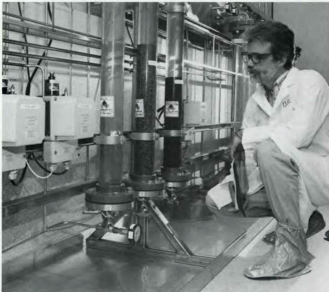
Tim Kent inspects purification columns used to remove hazardous materials from wastewater at the Wastewater Treatment Test Facility. This laboratory-in-a-trailer enables researchers to test and refine treatment techniques on a small scale before beginning full-scale operations.
