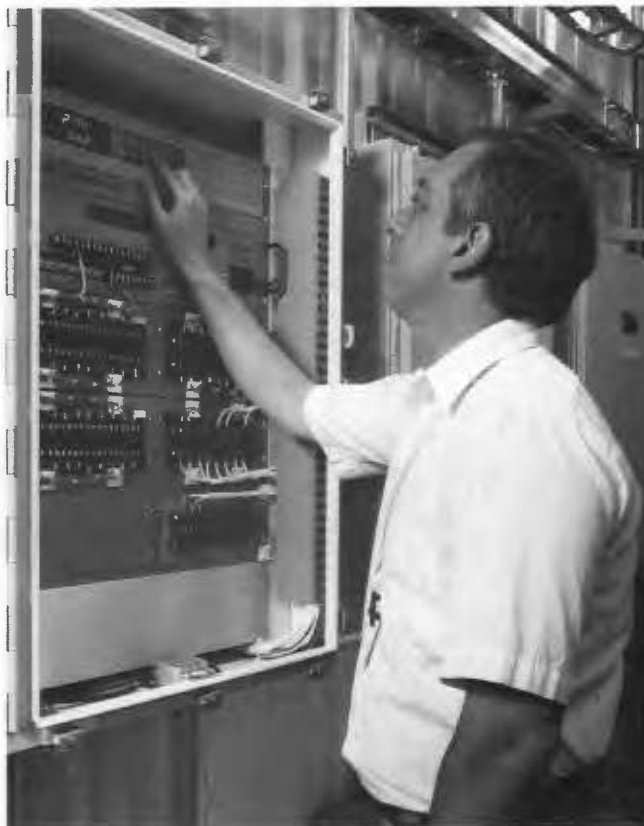
Andre Desjarlais can choose from a range of weather conditions when programming the Rotatable Climate Simulator.
