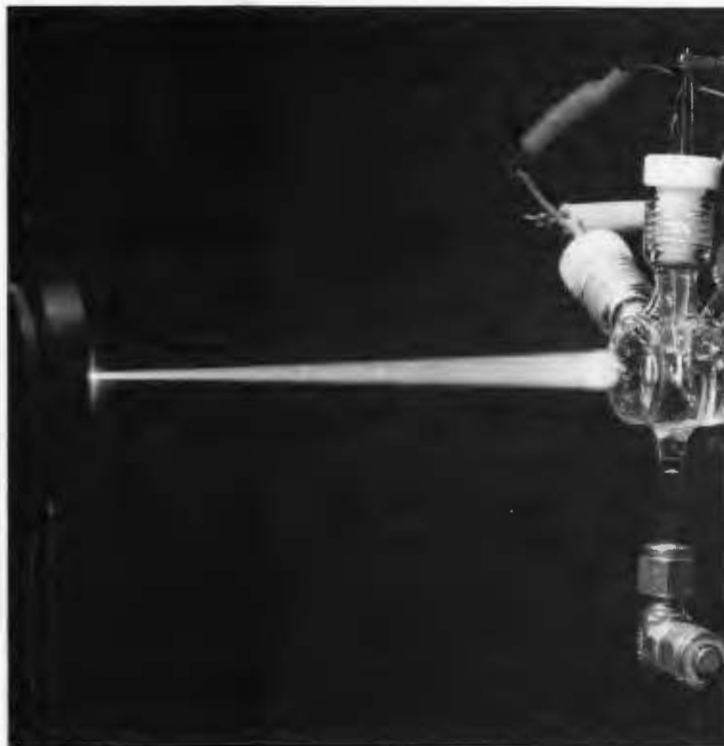
Closeup of the laser beam and the spectroelectrochemical sensor.
