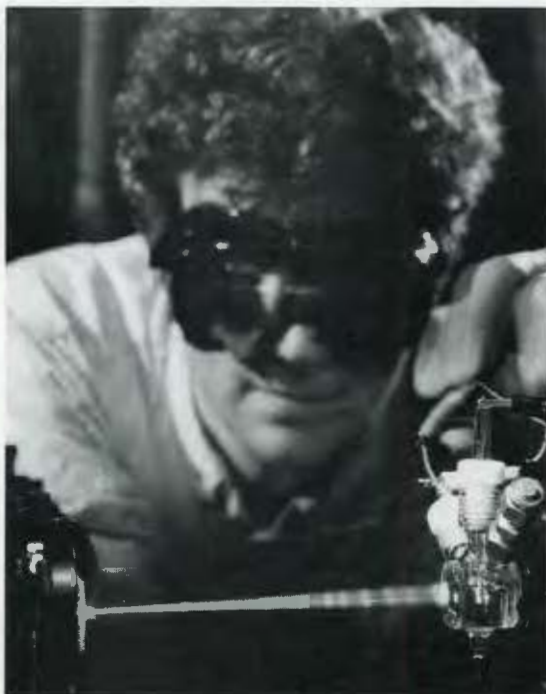
John Storey checks the krypton laser that is critical to the operation of the ORNL-developed spectroelectrochemical sensor for detecting and measuring groundwater pollutants.
