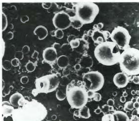
These "PacMan particles," so named for the holes on their surfaces, are formed by precipitation of hydrous aluminum oxide inside droplets during the transport of ammonia from the continuous to the dispersed phase.
