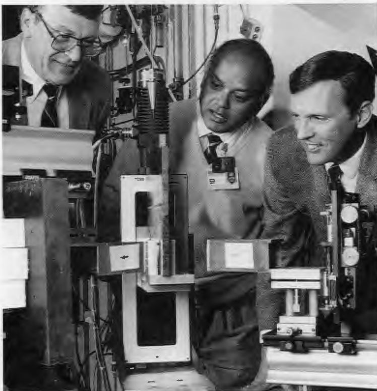
Steve Spooner (left), Stan David, and Cam Hubbard observe a welded sample whose residual stresses were characterized using neutron beam scattering. The arrows show the direction in which the neutron beam was passed. These ORNL researchers were members of a team that was first to measure residual stresses in a multipass weld, using a neutron beam from ORNL's High Flux Isotope Reactor.
