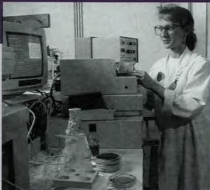
A spectrophotometer is used to screen contaminant-enriched bacterial cultures. Only one in every 50 cultures exhibits enough metabolic activity to require more definitive gas chromatography testing.
