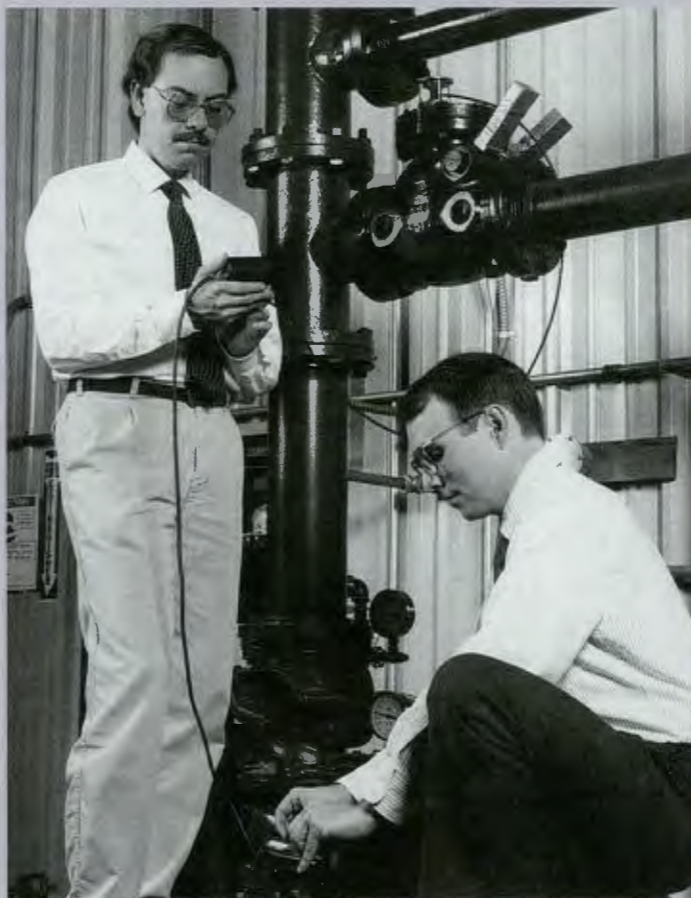
Howard Haynes (left) and Don Casada observe the performance of a check valve installed in a test loop in the Engineering Technology Division using methods ORNL developed to unintrusively monitor valve performance and degradation. A prototypical magnetic field concentrator device is located on top of the valve.
