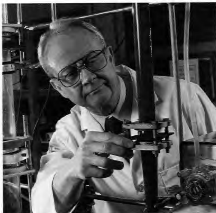
Chuck Scott examines a tapered column of gelatin beads containing microorganisms that could be used for removing contaminants or producing chemicals. Scott is director of ORNL's new Bioprocessing Research and Development Center.
