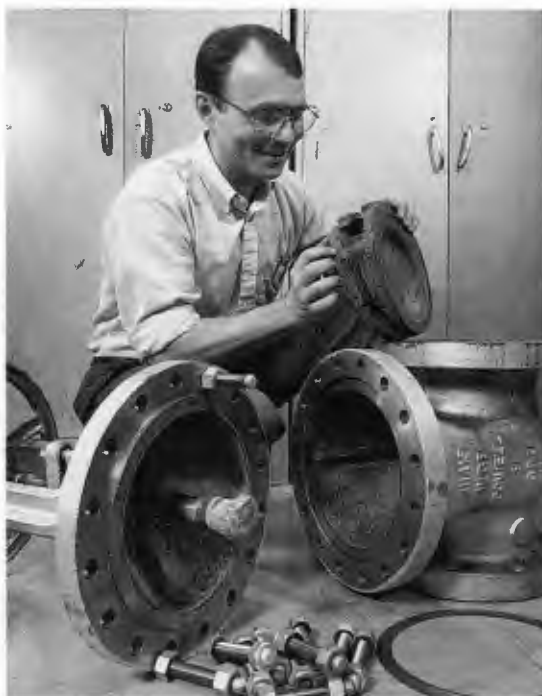
Don Casada examines a worn gate valve similar to valves used in nuclear power plants.
