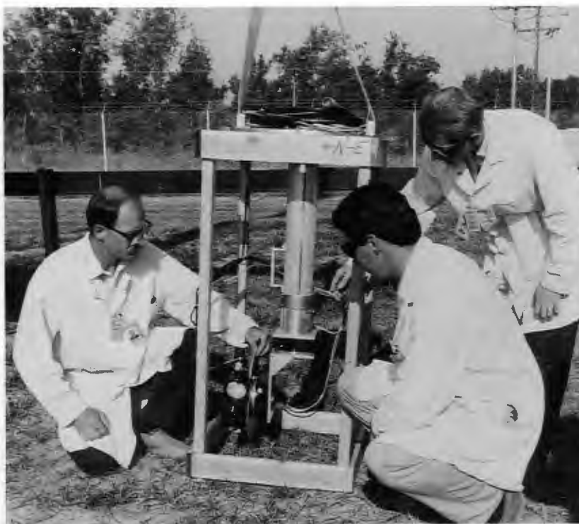
Barry Burks (left) of ORNL's Robotics and Process Systems Division and David Jacoboski and Dennis Nixon, both of the Westinghouse Environmental Management Company of Ohio, test the ORNL-developed automated surface-mapping system. It is being used here for the Fernald Environmental Management Project to obtain accurate data on the contour of waste surfaces. Such information was used to plan the cost-effective deposition of bentonite clay caps over the surface of radon-emitting uranium ore wasteforms.
