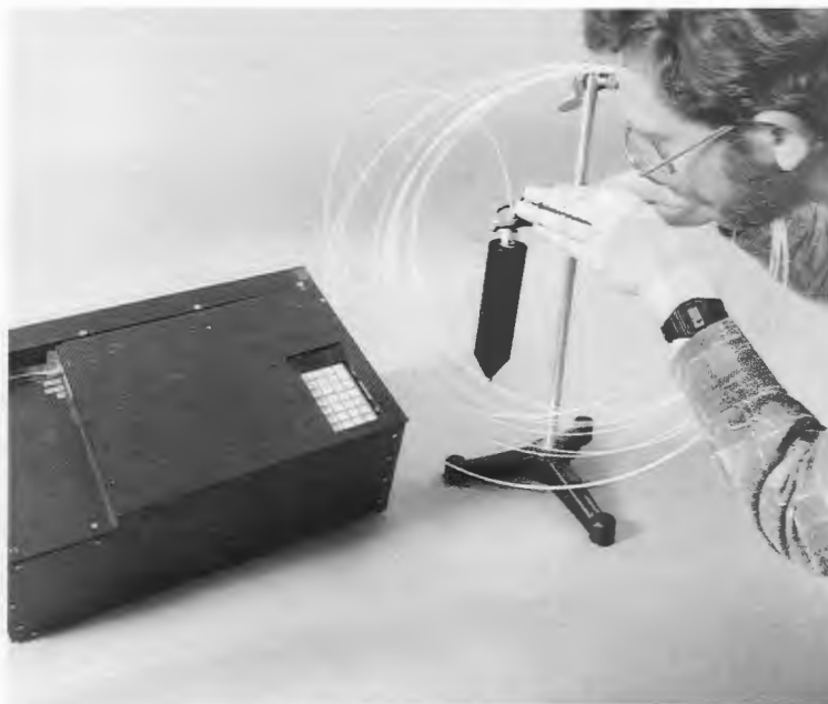
By detecting and measuring the concentration of groundwater contaminants directly, rather than by "sniffing" the air above the water, the DUVAS system, displayed here by John Haas of the Health and Safety Research Division, is able to more accurately characterize groundwater contamination.
