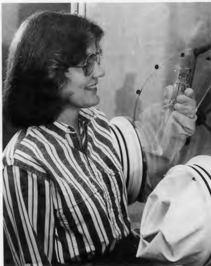
Nancy Dudney examines a thin-film lithium battery in the protective atmosphere of a glove box.
