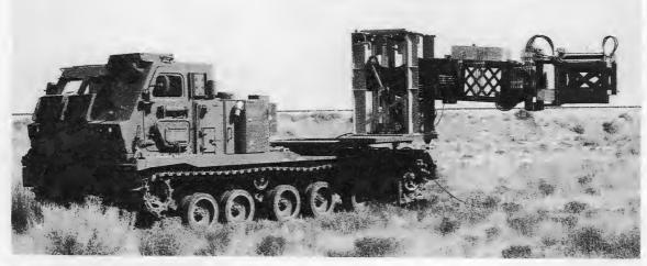
The FARS armored chassis has been fitted with the ammunition transfer arm and adjoining systems. The ammunition handling carousel and other FARS hardware and controls will be installed and integrated at ORNL.
