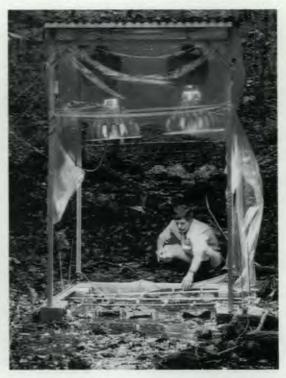
Pat Mulholland checks an experiment on the effect of increased light on stream algae in Walker Branch.
