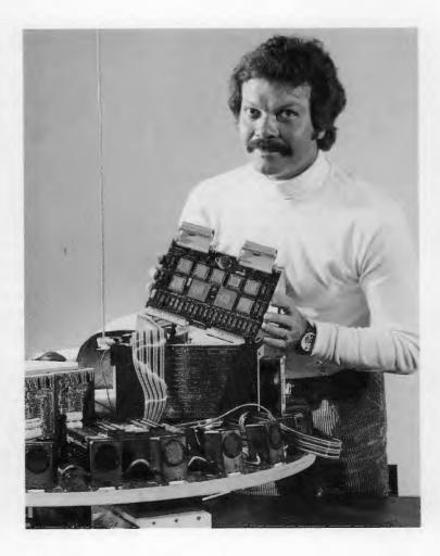
Francois Pin removes the seven-chip fuzzy logic control system from its slot on the mobile robotic platform. The cube-shaped objects ringing the platform are acoustic sonar sensors the robot uses to navigate.
