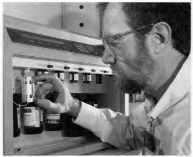
Bob Foote places a glass sample plate into the synthesis cell of a DNA synthesizer. The synthesizer manufactures specific sequences of DNA bases for use in hybridization research.
