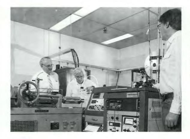
Bob Mesmer (left), Hank Cochran, and Mike Simonson inspect the feed system of the hightemperature flow calorimeter used to study the properties of supercritical aqueous solutions.
