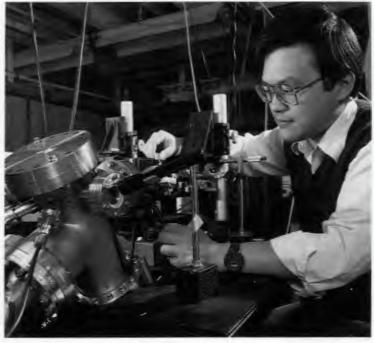
Kai Tang, a doctoral student in physics from Vanderbilt University, adjusts the optics of a laser used to vaporize DNA segments in the mass spectrometer's sample chamber.
