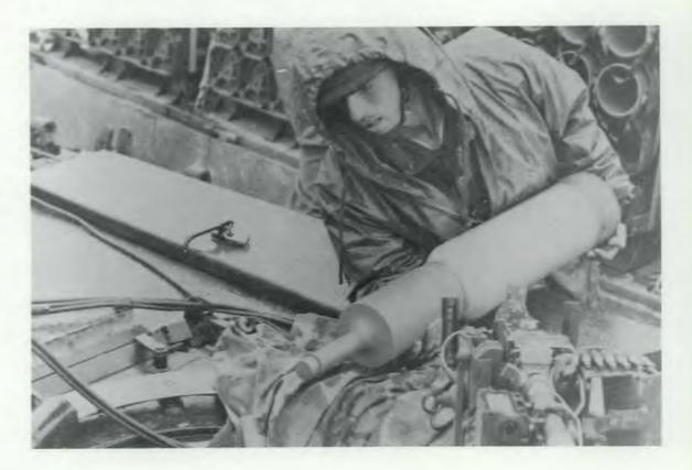
Ammunition is currently loaded by hand one piece at a time through the tank's hatch. This laborintensive activity exposes soldiers to weapon fire and nuclear, biological, and chemical agents.
