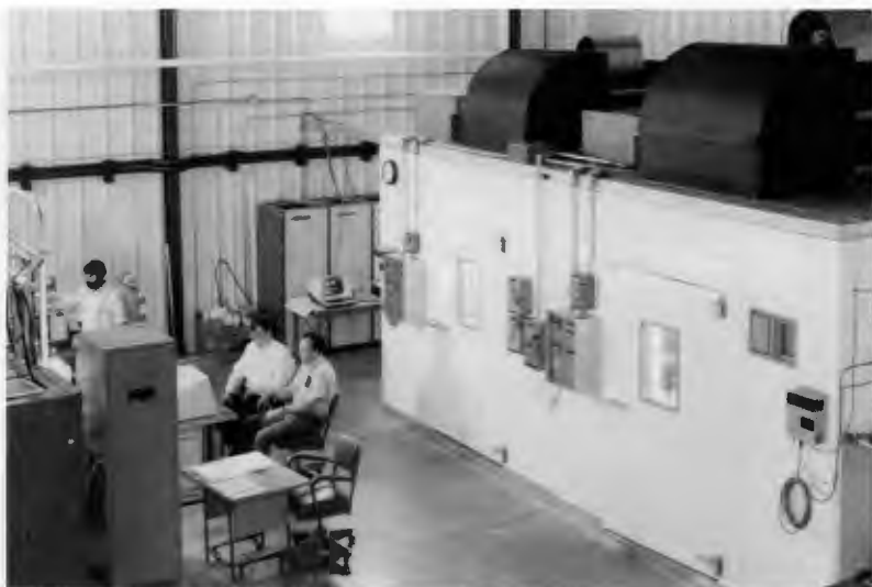
Ed Vineyard, Van Baxter, and Charlie Hardin observe results from tests of alternative refrigerants in the Building Equipment Laboratory. The large chamber in the center of the picture was used for testing several alternative refrigerants in a household refrigerator-freezer.
