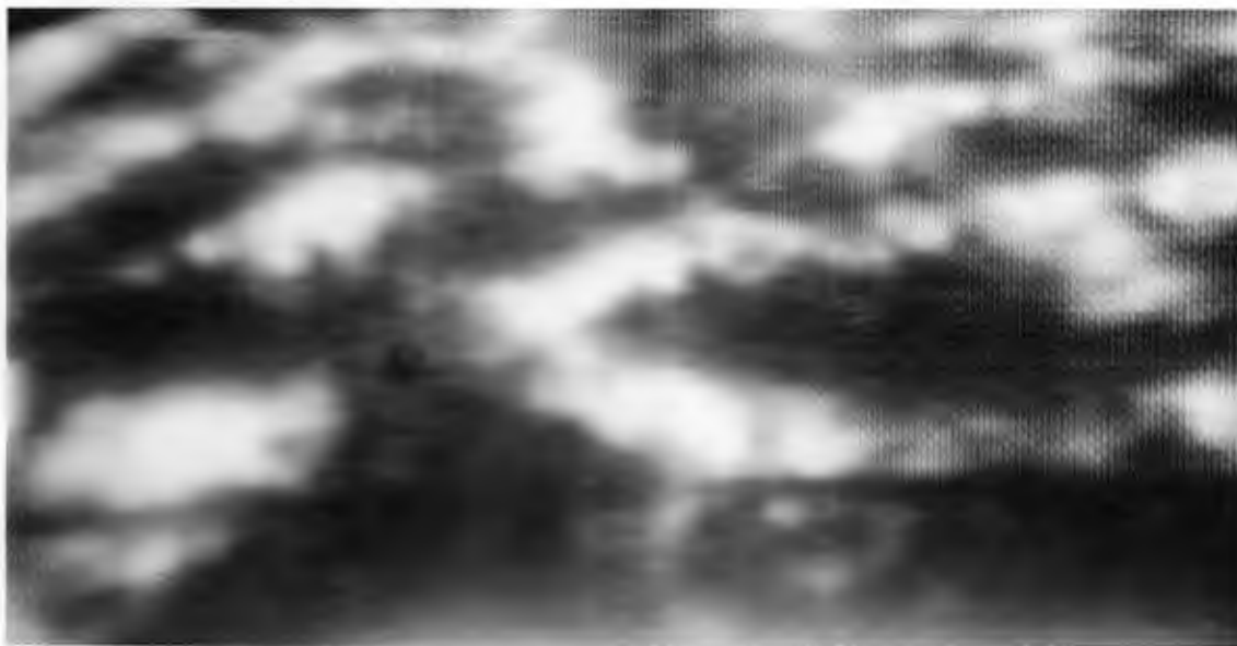
This photograph taken by an infrared camera shows the top surface of insulation in an attic having a temperature of -20^{\circ}\text{C} ( -5^{\circ}\text{F} ). The light areas in this hexagonal pattern are warmer than the dark ones.
