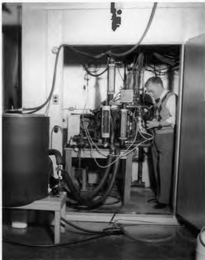
Jim Sand makes adjustments to the Alternative Refrigerants Calorimeter Facility, which is used to measure coefficients of performance and capacities of refrigerants.
