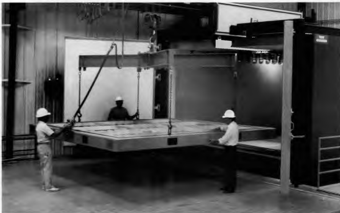
A crane moves test roof sections into the climate chamber of the $2-million Large-Scale Climate Simulator. The diagnostic platform, which can support a 10-ton panel, simulates a range of climatic conditions.
