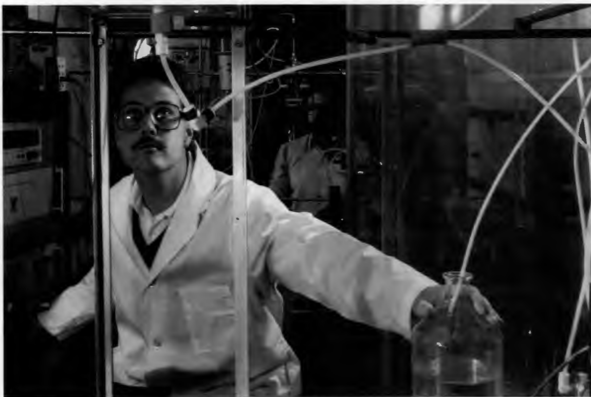
An ORNL-developed method for using high-intensity electric fields to control solvent-extraction processes improves performance efficiency 100 times while using only 1% of the energy required by devices now in use. Here, Timothy Scott (left) operates the electrically driven emulsion-phase contactor while Ron Brunson works with a related device, the electric-dispersion reactor.
