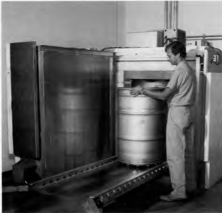
At the Waste Examination and Assay Facility, Don Coffey loads a drum of contact-handled transuranic waste into the passive-active neutron assay detector as part of the waste certification program.
