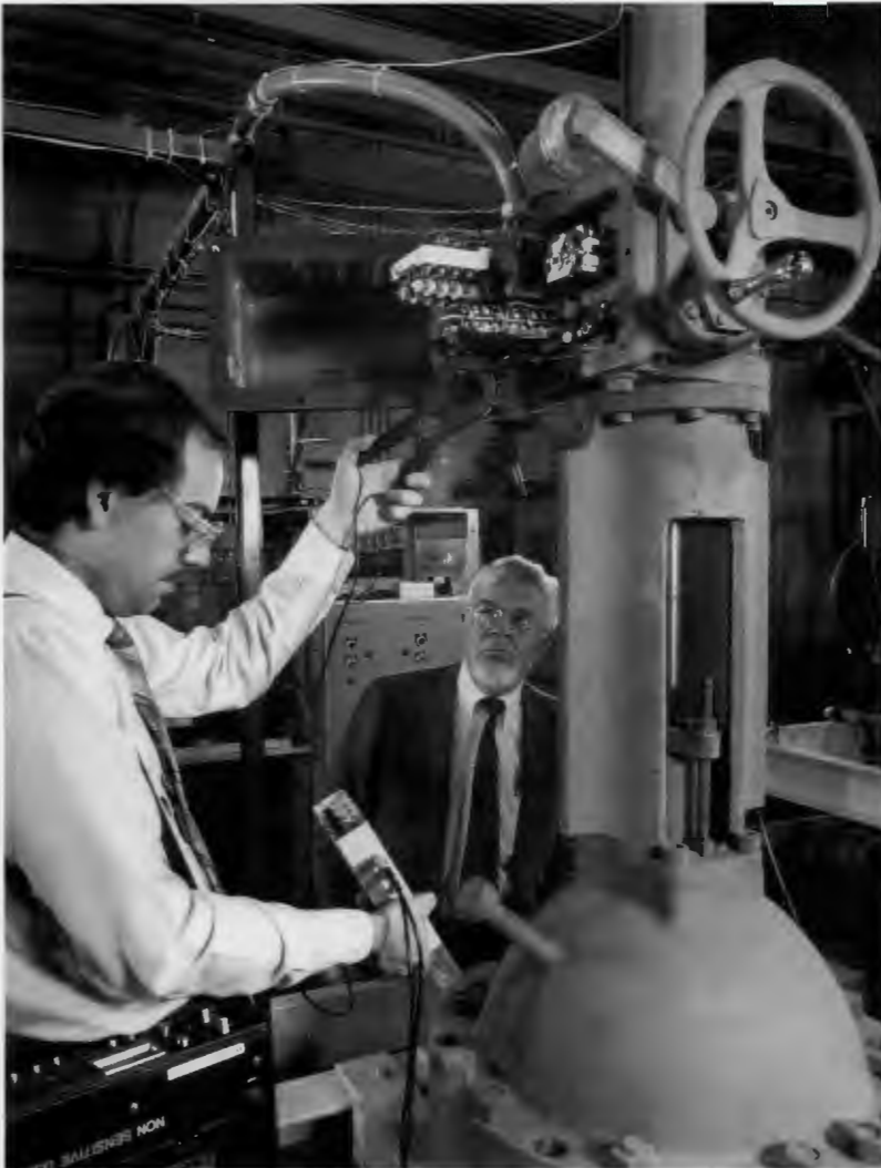
Howard Haynes (left) and David Eissenberg have developed a method for detecting mechanical and electrical abnormalities in a motor and the equipment it is driving. Here, Haynes attaches a clamp to wiring in a motor-operated valve as he and Eissenberg watch the signal conditioner current probe of a mobile motor current signature analysis device. The sounds are stored on a cassette tape for later analysis by the recorder Haynes is carrying on his shoulder.
