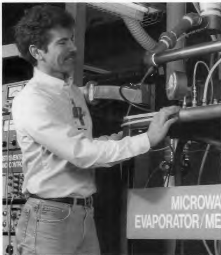
Terry White inspects his one-third-scale microwave processing experiment that dries and solidifies a 4.5-L can of simulated nonradioactive sludge.
