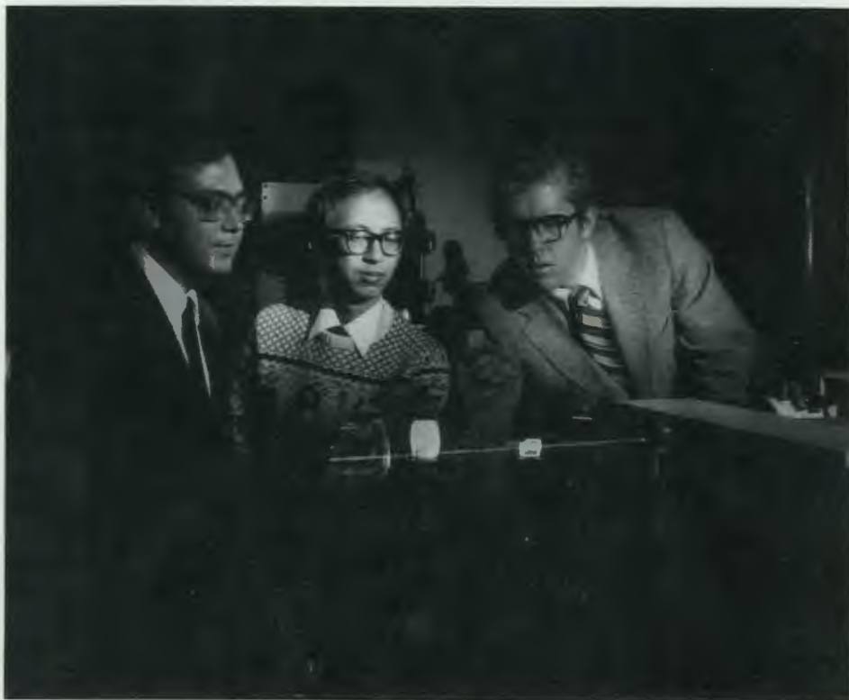
ORNL researchers have shown that clear alkali-halide crystals can monitor laser beams. The color tracks produced when the laser beam passes through the crystal give a three-dimensional profile of the beam and measure its divergence. No expensive instrumentation or computer printout is required. Developers are, from left, Steven Kramer, Chung-Husan Chen, and Michael McCann of the Health and Safety Research Division.
