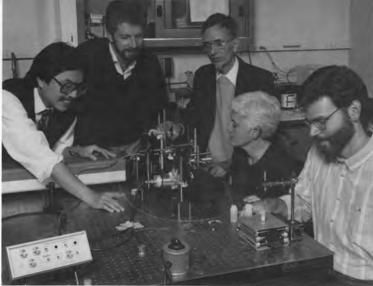
This laser-based detector sensitively and selectively measures human exposures to trace levels of hazardous environmental chemicals and infectious agents. Fibers as thin as human hair are used as a kind of "smart catheter" to analyze samples inside as well as outside the body. Members of the development team, from ORNL's Health and Safety Research Division and the Chemistry Department of the University of Tennessee at Knoxville, are, from left, Tuan Vo-Dinh, Michael Sepaniak, Guy Griffin, Kathy Ambrose, and Bruce Tromberg.
