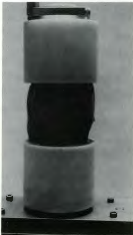
These concentric cylinders of gelatin and agar served as a soft-tissue-mimicking target in a large tank of water at the University of Rochester. A pioneering experiment using this target showed that ultrasonic diffraction tomography can be used to image soft-tissue inclusions such as tumors.
