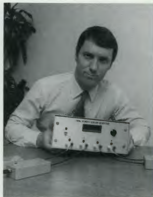
Bruce Jatho and team members from ORNL's Instrumentation and Controls Division developed an integral passive electronic circuit that simplifies the design and installation of large-scale control systems requiring many cables for connecting transducers and actuators. The device, which could be miniaturized as an integrated circuit chip, is used as a part of connectors or terminal blocks to identify wire-pairs and remote sensors.
