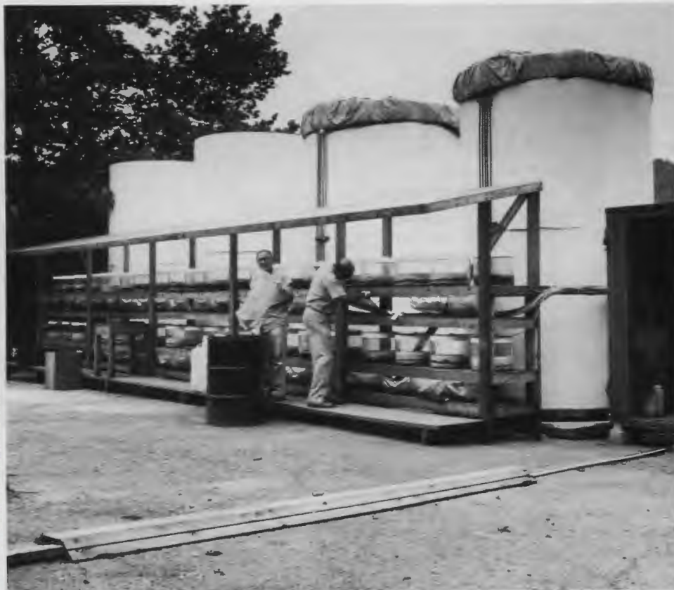
C.J.C. Gouch and O.M. Sealand of ORNL's Environmental Sciences Division check the results of a field test in which industrial wastes are leached with municipal waste leachate. The test helped to validate ORNL's new Toxicity Characteristic Leaching Procedure for identifying potentially hazardous wastes. EPA has proposed using the ORNL test for classifying wastes at municipal landfills and Superfund sites.
