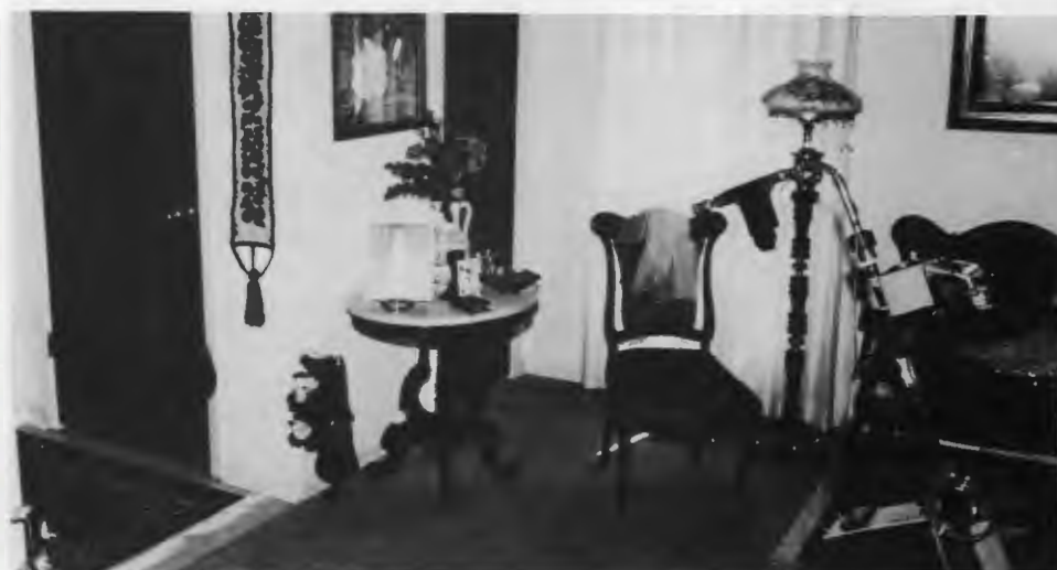
Equipment in living room (right) samples for the by-products of the decay of radon, which are health hazards. The passive samplers on the table measure average concentrations of various indoor pollutants.
