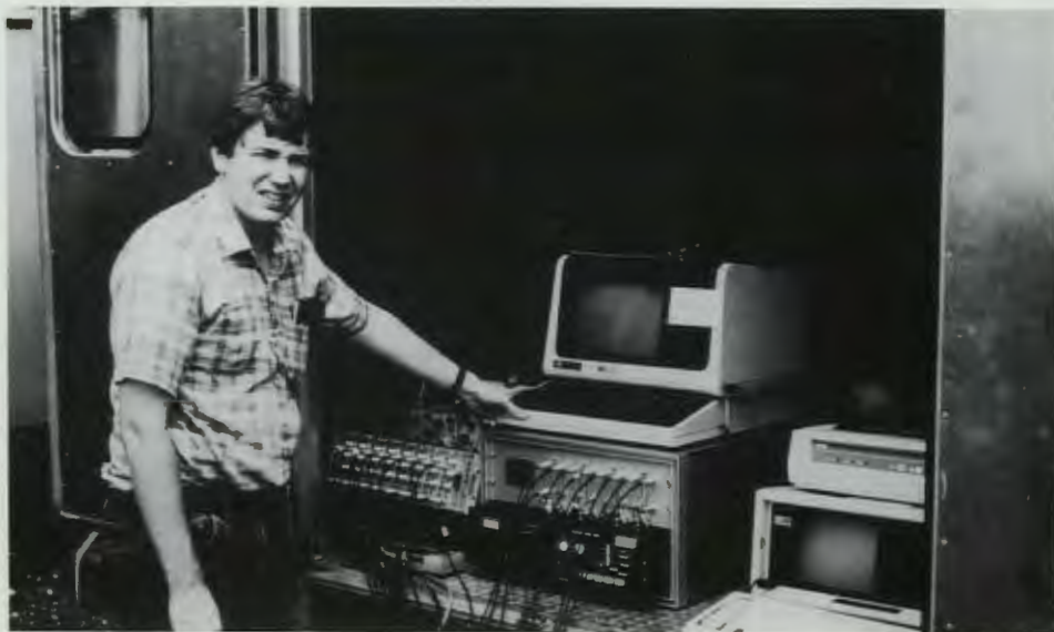
G. R. Wetherington, Jr., of ORNL's Instrumentation and Controls Division checks the operation of the Fast Data Acquisition System. The system is used in the Athens Distribution Automation and Control Experiment to determine the effects of control actions on distribution feeders.
