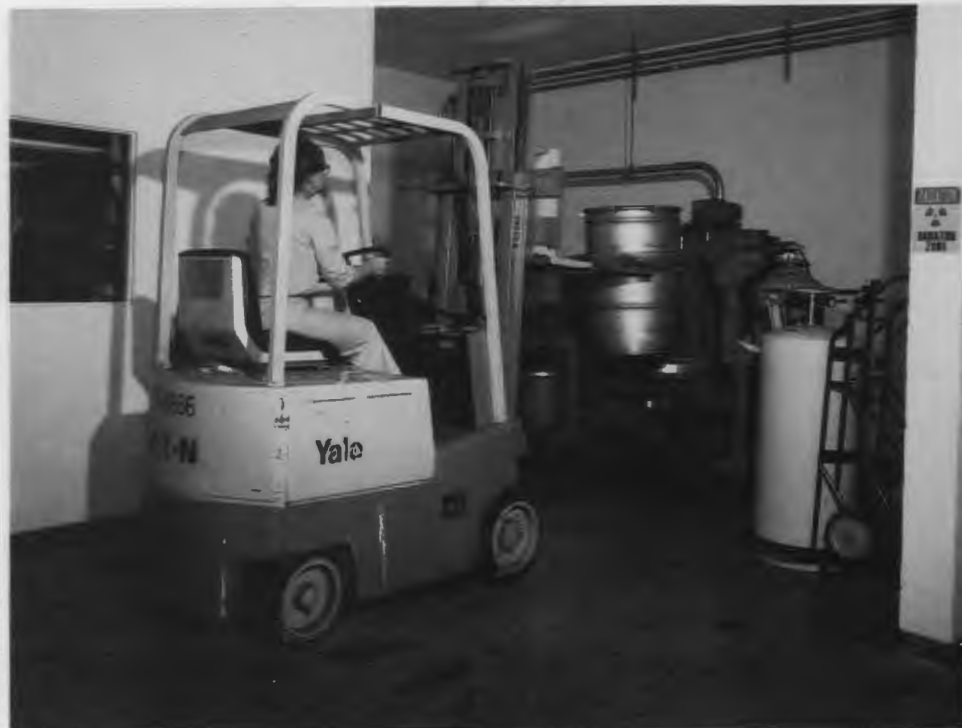
Babette Norris, technician at ORNL's Waste Examination Assay Facility, loads a waste drum onto the drum turntable of the segmented gamma scanner, which is used to help identify and quantify any transuranic wastes in waste drums.
