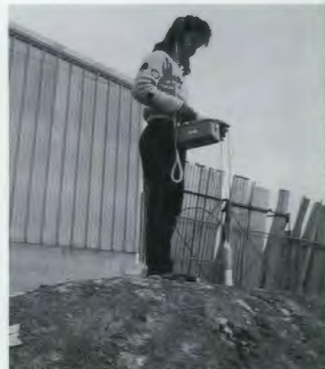
Gretchen Smith uses a gamma scintillation detector to survey the property outside a Grand Junction warehouse.
