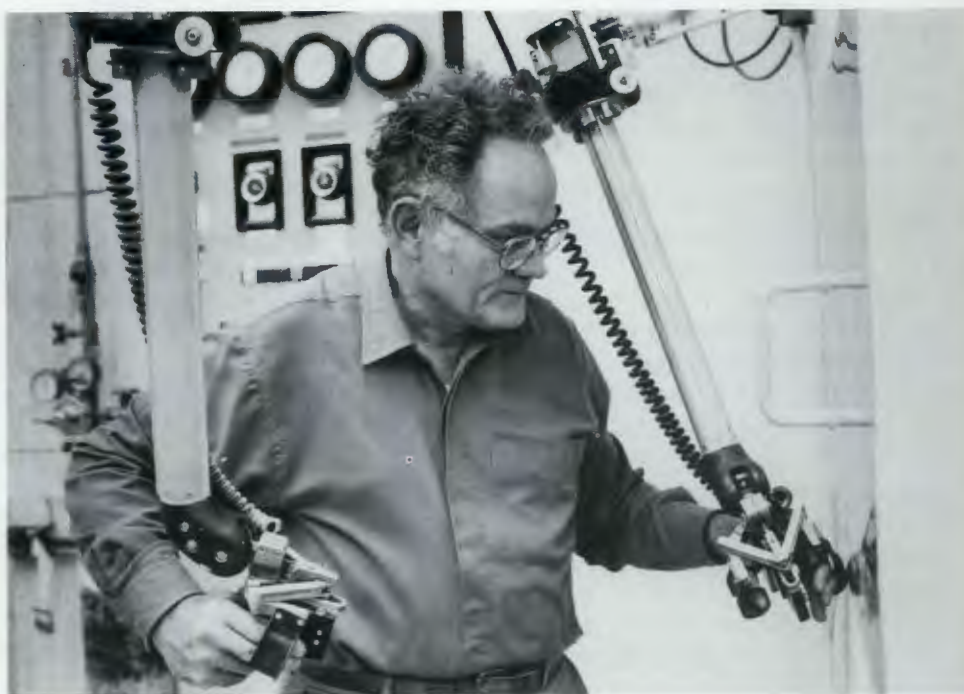
Frank Dyer operates remote manipulators in the HFIR neutron activation analysis laboratory.
