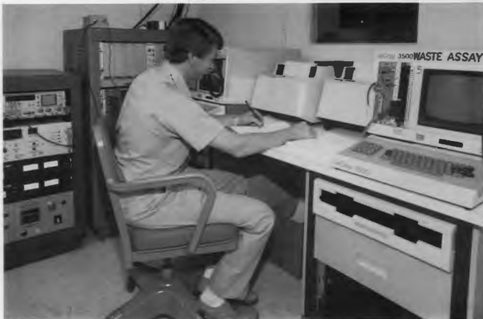
The transuranic Neutron Interrogation Assay System developed at Los Alamos National Laboratory is so sensitive that it can detect 1 mg of fissile material in a transuranic (TRU) waste mixture filling a 208-L (55-gal) drum. It is capable of performing rapid, quantitative assays of wastes and scraps having a low fissile content that are contained in high- or low-density matrices. A computer operates the entire system. Here Don Coffey, ORNL technician, enters TRU waste assay data into a log book.
