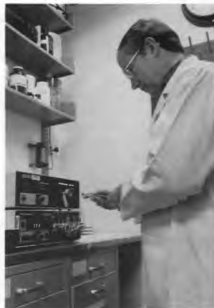
Gary Sega injects a sample of hydrolyzed DNA into a high-performance liquid chromatography (HPLC) system. The DNA was recovered from mouse germ cells exposed in vivo to labeled ethylene oxide gas. The HPLC system can separate various DNA adducts produced by different chemical mutagens.
