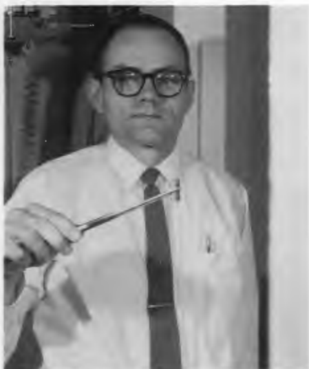
Dyer holds a plastic rabbit used for irradiations of samples in the High Flux Isotope Reactor.
