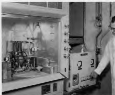
Juel Emery checks the rabbit tube control panel in preparation for a neutron activation analysis measurement.
