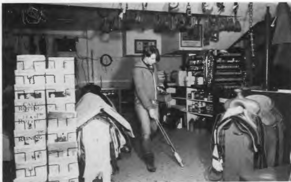
Kathy Dickerson, ORNL field team leader, uses a hand-held radiological monitoring device to detect radium in the foundation of a Western-wear shop in Grand Junction. Uranium-ore mill tailings were used as a construction material on private and public properties.
