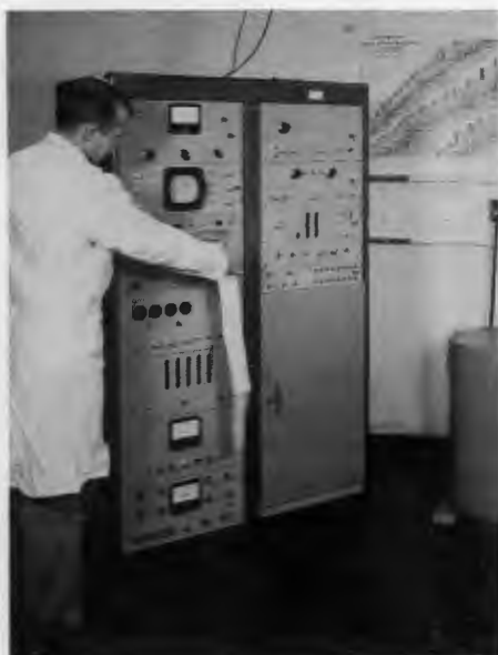
Ed Strain examines data from a 200-channel, vacuum-tube analyzer, which acquired gamma spectra for NAA until 1964. The same type analyzer was used in the Kennedy assassination probe carried out at the Laboratory (see following article).
