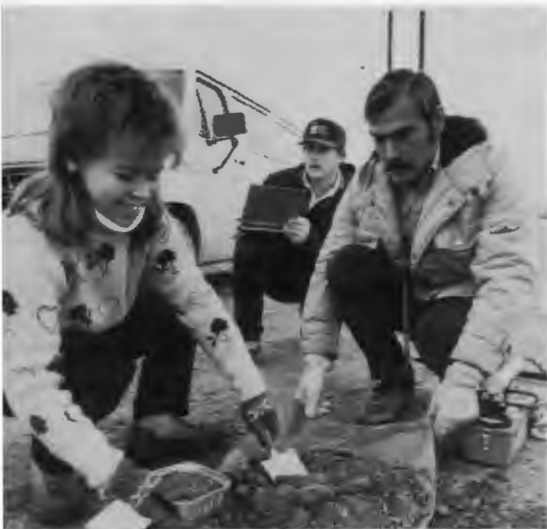
A HASRD Radiological Survey Activities team collects a soil sample in Grand Junction during a radiological survey for DOE's Uranium Mill Tailings Remedial Action Project. Team members are, from left, Gretchen Smith of ORAU, Chris Muhr of ORNL, and Mike Roche of ORAU. The project has evaluated about 3000 properties for the presence of uranium-ore mill tailings.
