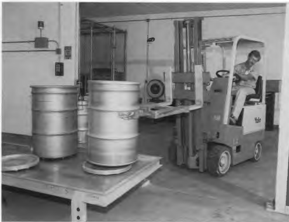
Operating a fork lift, Coffey loads a TRU waste drum onto a drum-loading platform where its waste contents will be measured by the Neutron Interrogation Assay System.
