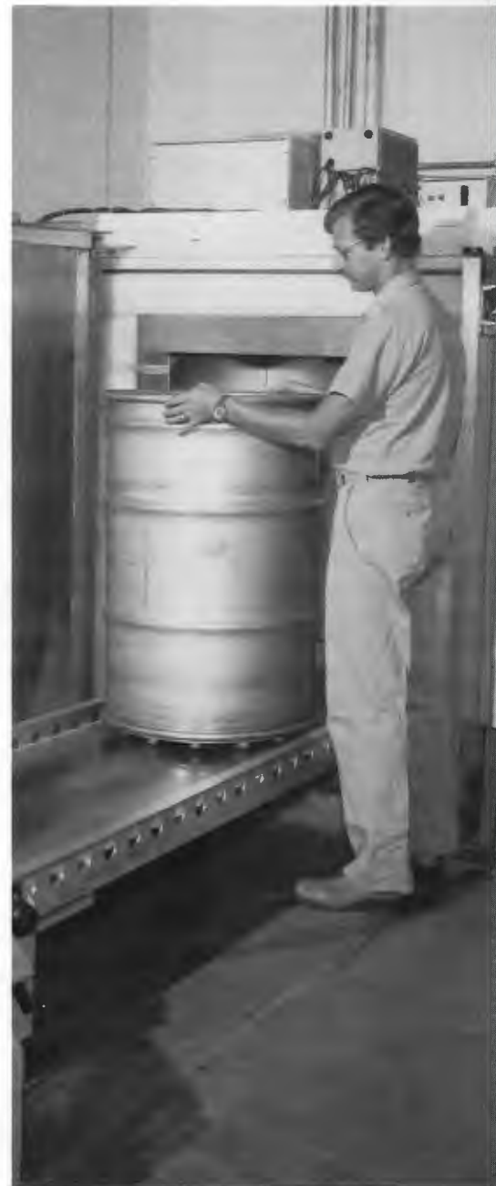
Coffey loads a TRU waste drum into the Neutron Interrogation Assay System. Part of this system consists of a gamma-ray drum scanner, which can detect and measure gamma-ray-emitting isotopes in 208-L (55-gal) drums filled with low-to-medium-density wastes such as rags, towels, rubber gloves, and similar material.
