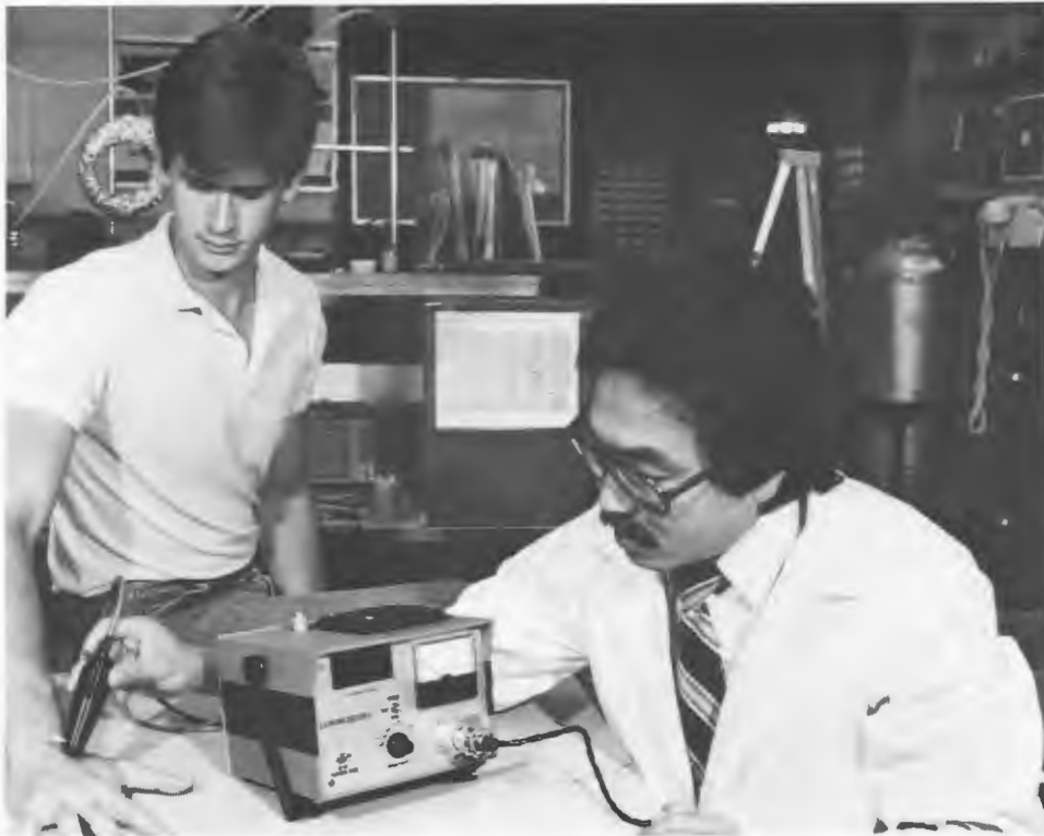
Tuan Vo-Dinh (right) uses the fiber optics luminoscope that he developed to check whether D. A. White's hand is contaminated. This instrument, now being manufactured by Environmental Systems Corporation in Knoxville, can monitor the skin of workers who are exposed to oil and tar materials containing potentially carcinogenic compounds.
