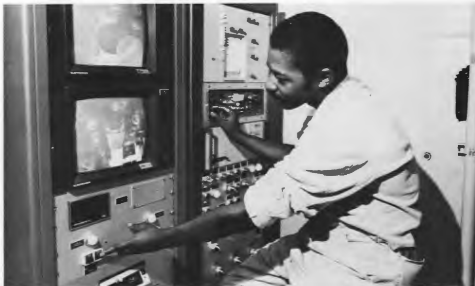
Randy Kirk controls a remotely operated welder to seal a CEUSP can before storing it for a long time. This procedure is performed remotely because the solidified uranium inside the can is highly radioactive.
