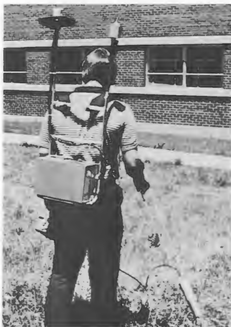
Mike Blair demonstrates USRADS by conducting a radiological survey of an area near Building 3500 at ORNL.
