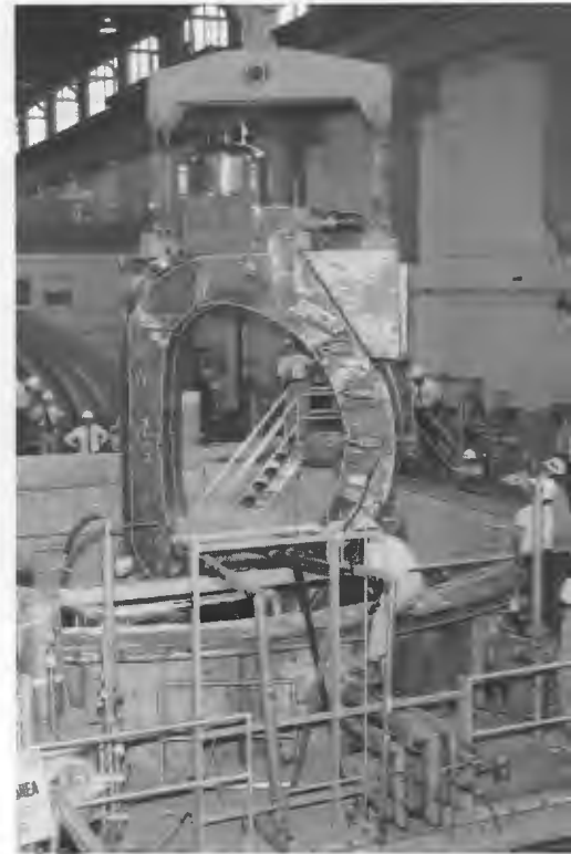
The General Dynamics coil (shown here), along with the Japanese coil, was subjected to an early test in the summer of 1984. Tests on both coils were successfully carried out to the full design current of 10,000 amperes.
