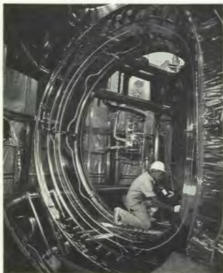
THE COVER: Craftsman Maurice Love checks out the superconducting magnet made in Japan and now being tested in an international facility at ORNL. The story behind the six magnetic coils in the facility is told in the article on page 30.
