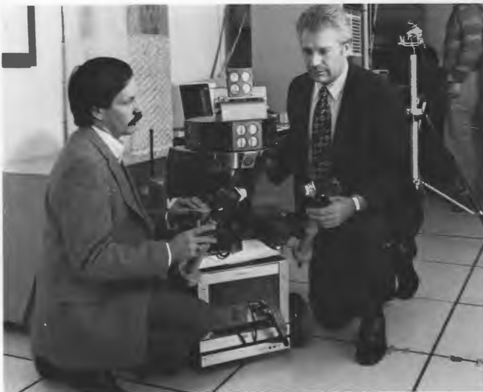
Bill Hamel (left) and Chuck Weisbin examine the HERMIES-II robot, which is used by the Center for Engineering Systems Advanced Research for concept demonstration of artificial intelligence planning and learning algorithms.
