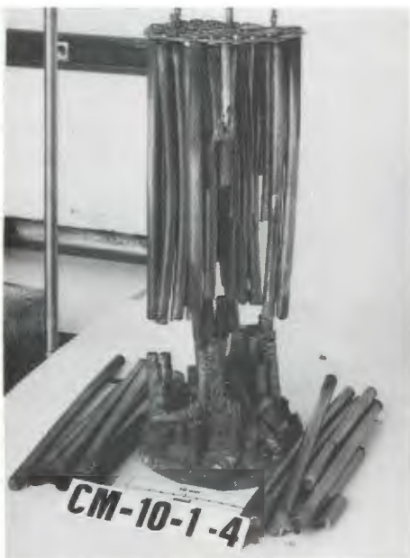
This experiment in the Core Melt Facility had graphic results. A bundle of uranium-oxide fuel rods was heated to 1800°C in the facility. As a result, the Zircaloy-clad fuel bundle was partially degraded, and "run-off candling" of a silver-alloy-Zircaloy intermetallic phase is evident at the bottom.
