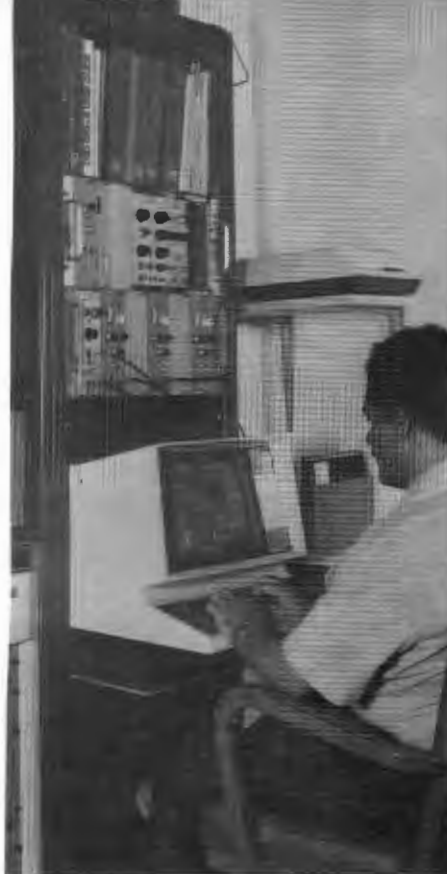
Charlie Webster operates the multichannel analyzer and gamma detector to identify and quantify fission products released from irradiated segments of fuel rods similar to those used in light-water reactors.
