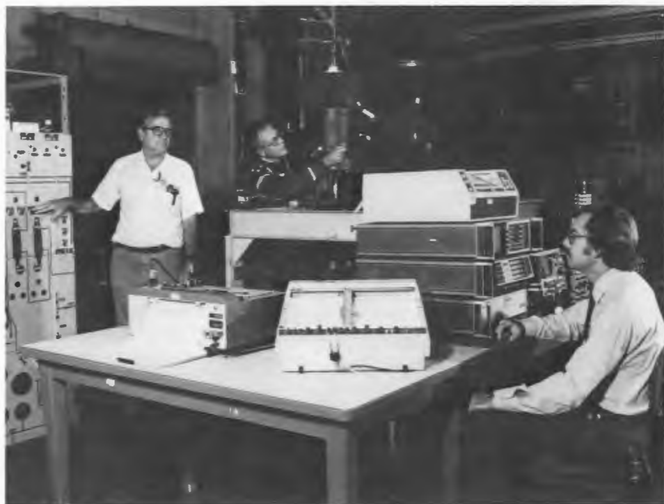
E. L. Biddle (left) and H. D. Haynes (right) of ORNL's Engineering Technology Division and R. C. Kryter of the Instrumentation and Controls Division are evaluating the diagnostic capabilities of a variety of sensors for motor-operated valves. This study will lead to improved methods for detecting age-related defects and monitoring wear over time in motor-operated valves in nuclear power plants.
