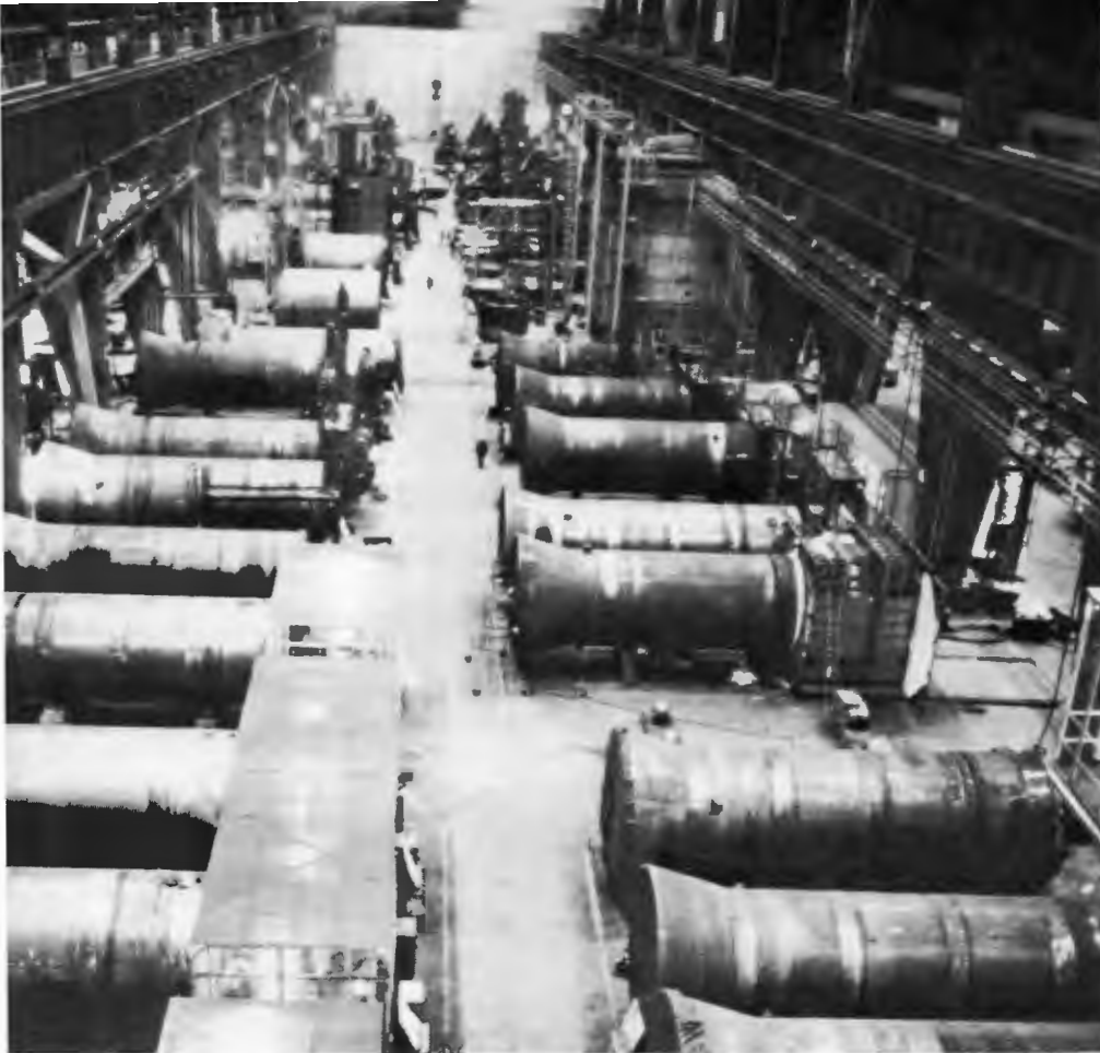
Steam generators for French nuclear power plants are manufactured in Framatome's facility.
