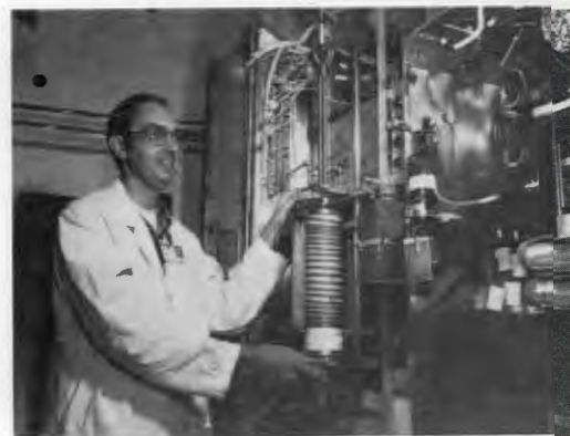
James R. Travis checks ORNL's vertical furnace fission product release apparatus used to study the chemical fate of fission products from fuel rods under accident conditions.
