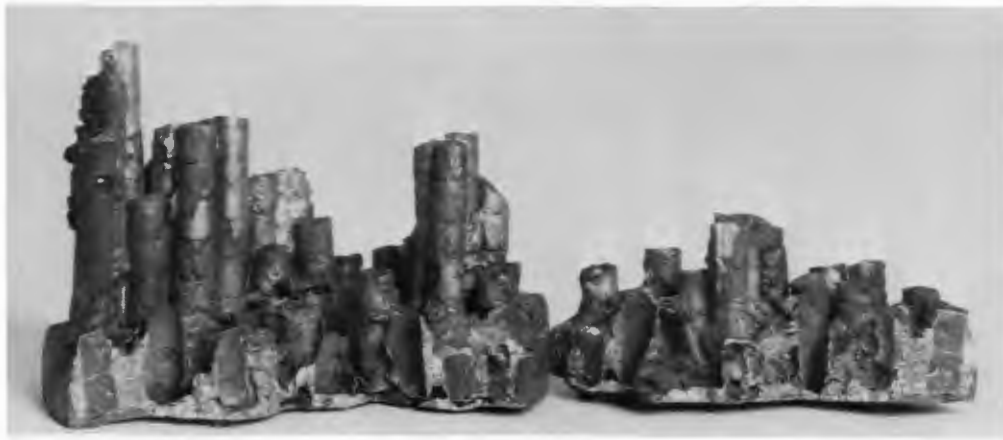
This recovered intermetallic residue from the base of the melt residue is an extremely hard material typical of what might be found after a core-damaging accident such as that at Three Mile Island. This low-melting eutectic is formed by reaction of stainless steel in the fuel cladding with Zircaloy in the surrounding sheath. ORNL's observations of melted core materials could affect the design of tools for core removal at TMI.
