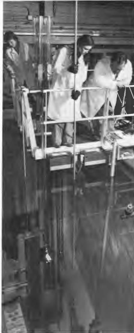
Technicians working from a bridge over the pool of the Oak Ridge Research Reactor adjust an experimental rig that extends through the top of the containment tank to the reactor core. All procedures are monitored carefully to prevent overexposure.
