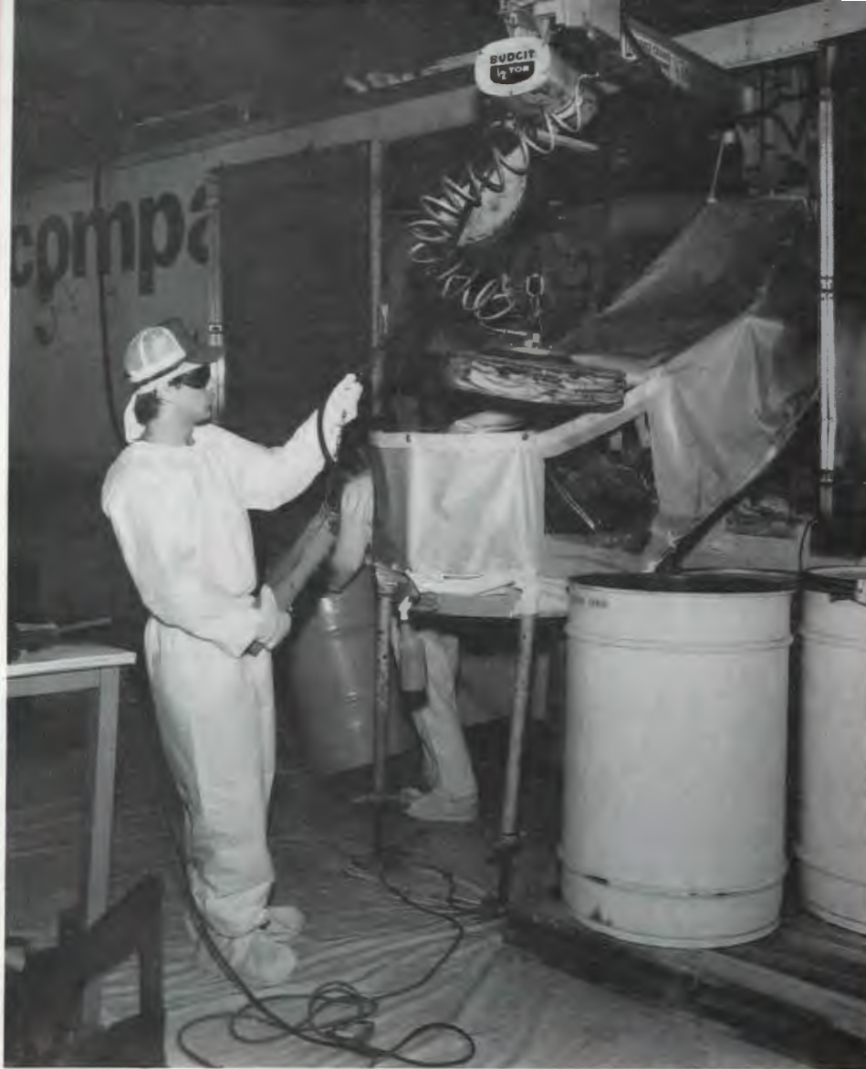
Using a small crane, a Westinghouse-Hittman technician removes a crushed steel drum for loading an overpack container to be stored in the ORNL burial ground.
