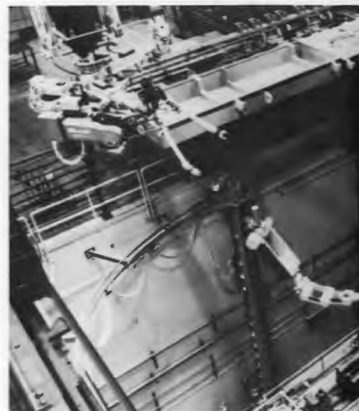
Remotely operated manipulators and transport systems at ORNL verify the feasibility of remote maintenance concepts. This prototypical fuel reprocessing equipment is located in the Remote Operations and Maintenance Demonstration area of the Integrated Equipment Test Facility.
