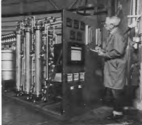
Vic Fowler, technician, checks the operation of the ion-exchange pilot plant designed and built recently by ORNL to reduce generation of low-level waste at the Process Waste Treatment Plant.
