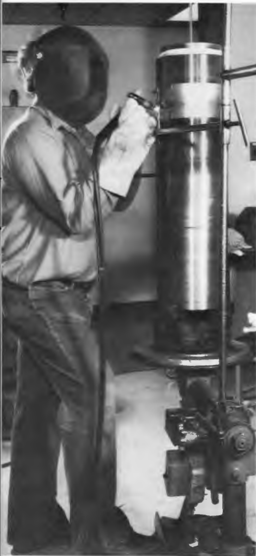
ORNL welder joins a pipe made of a modified chromium-molybdenum (9 Cr: 1 Mo) steel alloy to a type 304L stainless steel safe end before it is installed for a one-year test in the Sodium Components Test Loop at the Energy Technology Engineering Center in California. The center is operated by Rockwell International. The test loop is used to test liquid-metal reactor components. ORNL helped to develop the steel alloy.
