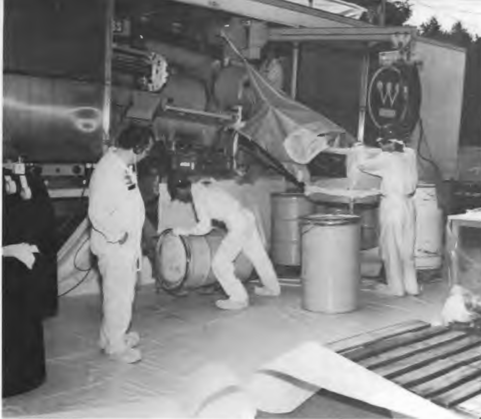
During a demonstration of a new low-level-waste-compaction system at ORNL, a Laboratory health physics technician watches as a Westinghouse-Hittman crew loads a drum of radioactive waste for insertion into the compactor.
