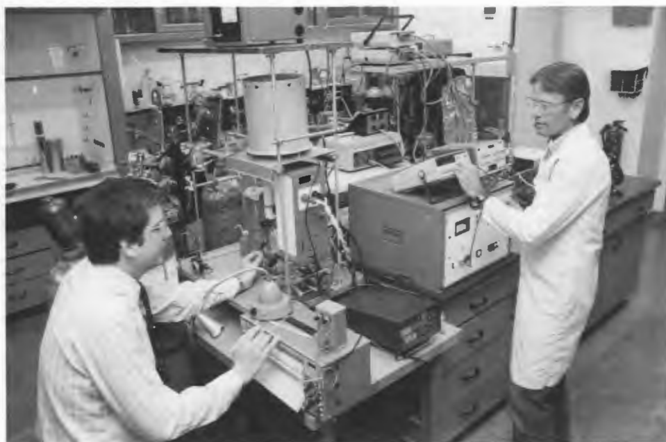
Mark Reeves (left) checks a cuvette that holds algae, which is exposed to light from the xenon flash lamp up front. Jim Thompson checks the power source that supplies electricity to the lamp. The two researchers have used this apparatus to measure photosynthetic unit sizes for hydrogen and oxygen production from living algae.
