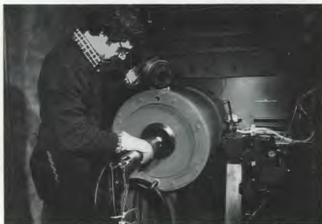
Mike Naney loads the furnace assembly and samples into the internally-heated pressure vessel. The apparatus is capable of heating samples to 1400°C at hydrogen pressures up to 500 MPa. Hydrogen gas is used in this facility to create a reducing atmosphere—that is, to remove oxygen from materials, permitting studies of oxidation-reduction dependent reactions that are important in natural magma systems.
