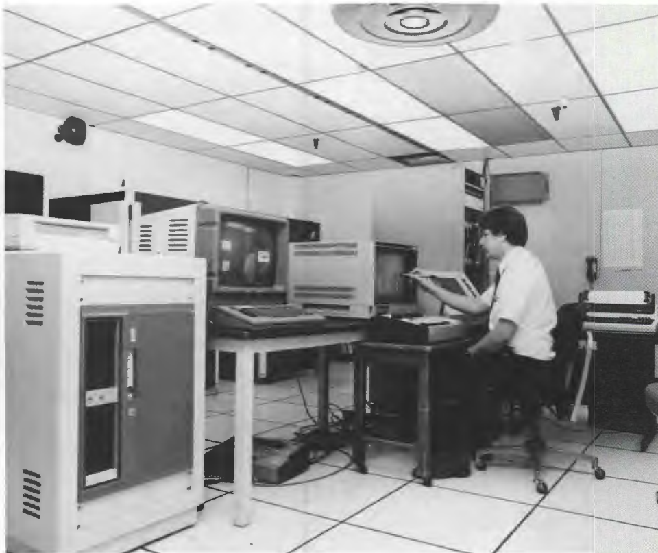
Randall Wetherington uses a light pen to call up information from the AACETS supervisory control and data acquisition (SCADA) system, which is based on a Digital Equipment Corporation PDP 11/44 minicomputer. The results of the electrical system simulation (performed by the smart test panel) are made available to the SCADA system through interfacing analog and discrete signals (exactly like those that will be present in Athens). The smart test panel sends the signals to the RTU, which digitizes them and telecommunicates the data for processing by SCADA real-time software. A larger SCADA system will be installed at the Athens Communication Control Center to monitor and control the Athens electrical system.
