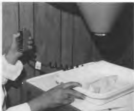
An experimental rat is positioned under ORNL's new gamma camera detector following the intravenous injection of a radioactive test compound to determine the distribution of radioactivity in the animal's tissue.
