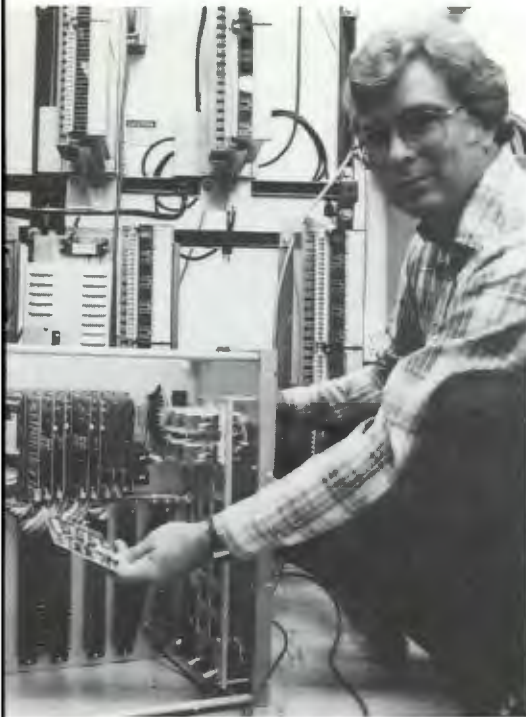
Jerry Bentz, an electrical engineer, checks out a remote terminal unit (RTU) at ORNL that is part of the Athens Automation and Control Experiment Test System (AACETS). It is similar to the RTUs to be installed in the Athens substation and on the distribution feeder that sends data to the Athens Communication Control Center.
