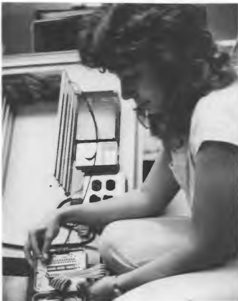
Eva Broadway, an ORNL electrical engineer, shows some components of a data system that will be installed in an Athens substation to gather preexperiment (characterization) baseline data on power consumption and weather variables. These data will be compared with data obtained during the experiment, which is designed to improve the distribution efficiency.
