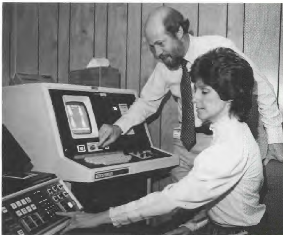
Linda Alley and Knapp operate the new gamma camera and computer system, which was recently acquired to evaluate the tissue distribution and kinetics of ORNL-developed radiopharmaceuticals in experimental animals.
