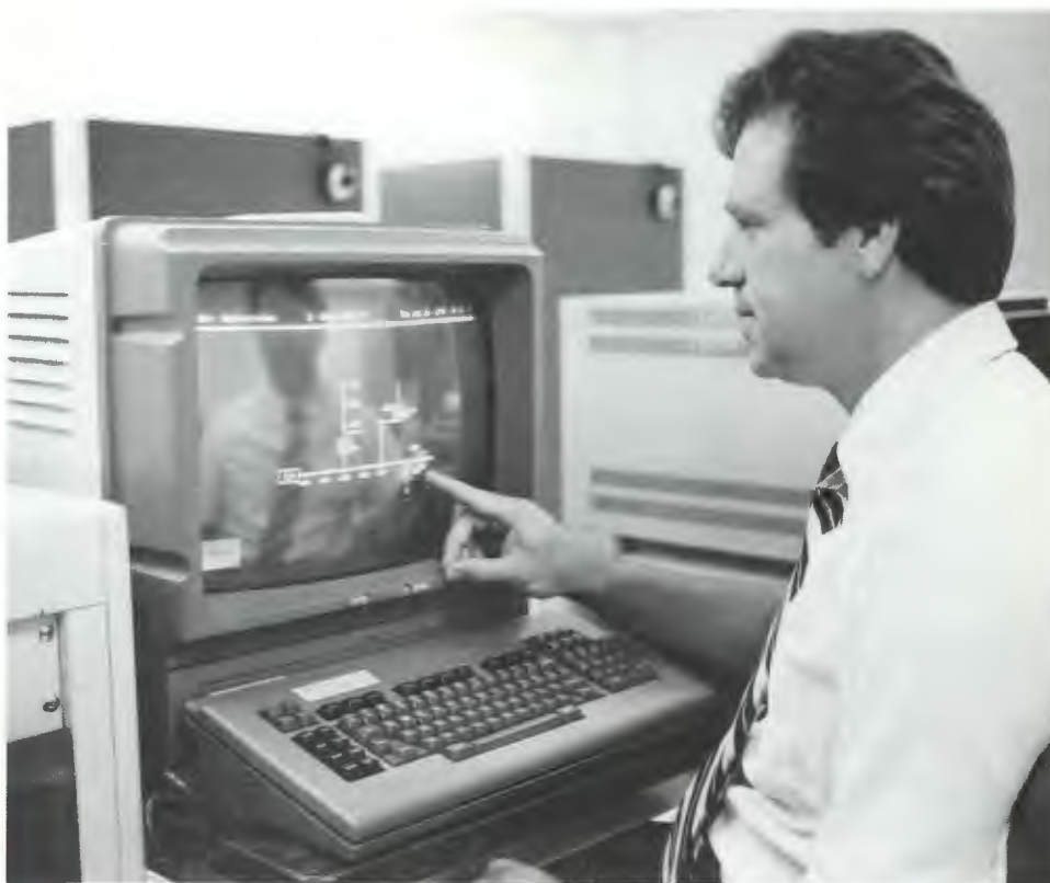
Purucker taps the touchscreen of the smart test panel (at ORNL's Instrumentation and Controls Division), which simulates the electrical system of the Athens Utilities Board. This smart test panel is part of AACETS, which will be used to develop the experimental control ideas into real-time software to be employed during the Athens experiment beginning in 1985.
