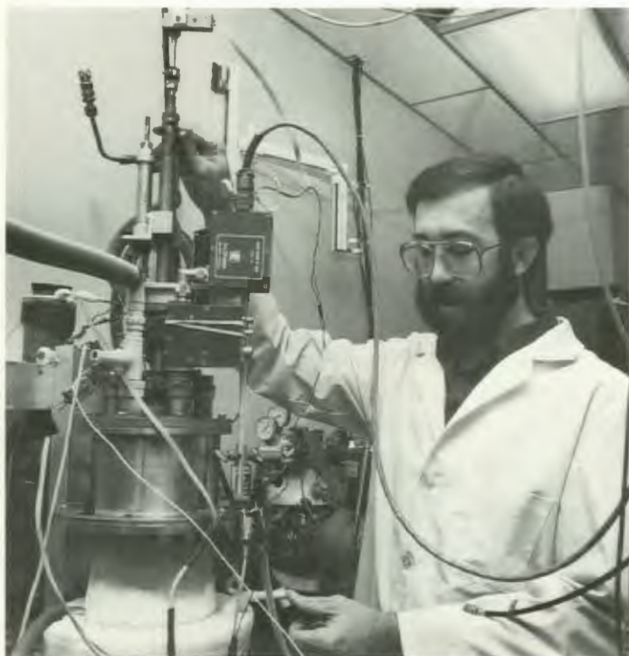
Stan Nave adjusts the micromagnetic susceptometer located at the Transuranium Research Laboratory. This highly sensitive instrument, which incorporates a superconducting quantum interference device (SQUID), is used to derive the magnetic behavior of transplutonium elements in samples as small as 1 microgram.
