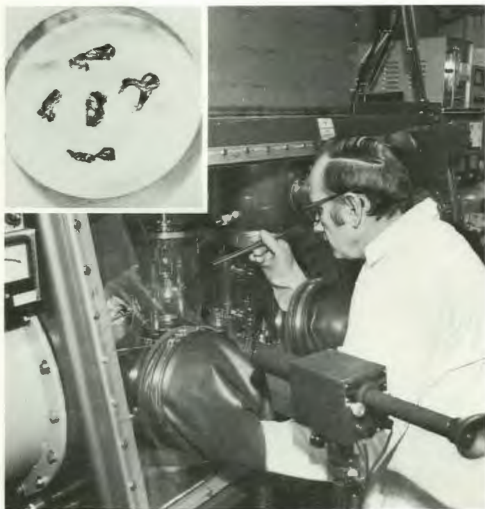
Dick Haire uses high-vacuum equipment in a helium atmosphere glove box to prepare 8 micrograms of berkelium metal. Berkelium was used in a collaborative research project with Los Alamos National Laboratory to measure the metal's enthalpy of sublimation. Inset: These pieces of berkelium metal on a 6-mm diam quartz disk were cut from a 8-microgram product prepared by reducing a berkelium-fluorine compound ( BkF_3 ) with lithium metal.
