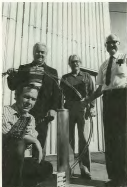
Ken Valentine, Manfred Kopp, George Guernant, and James Harter (left to right) display the ultrahigh-sensitivity fission counter that they developed. This neutron detector and its associated instrumentation were developed for neutron flux monitoring in the Clinch River Breeder Reactor Plant.
