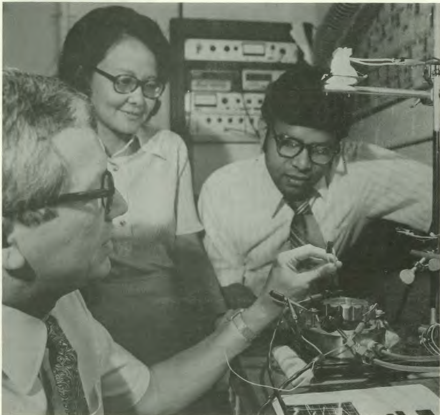
This solar cell being tested for its efficiency in converting simulated sunlight into electricity was developed at ORNL using a new laser technique.
