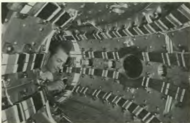
A view inside the ORMAK torus. This was one of the early tokamak experiments aimed at solving the physics problems of deriving vast quantities of energy from deuterium, an extremely abundant hydrogen isotope found in the ocean.
