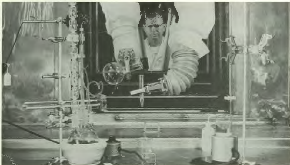
An ORNL technician uses remotely controlled manipulators in a hot cell to handle radioactive chemicals.
