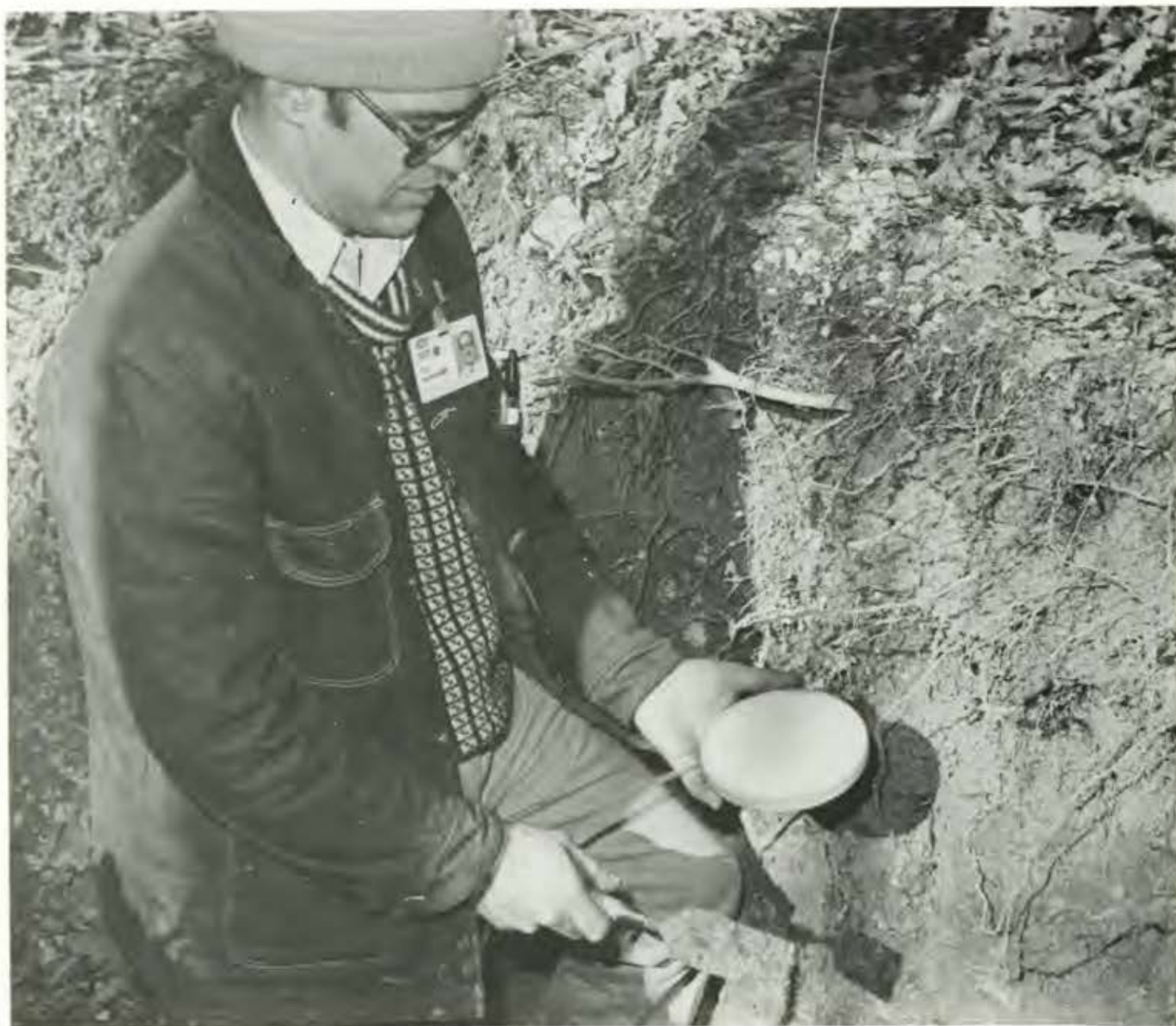
Dan Richter inserts a lysimeter plate to collect soil water for analysis. ORNL ecologists are studying the effects of whole-tree harvesting on forest productivity.
