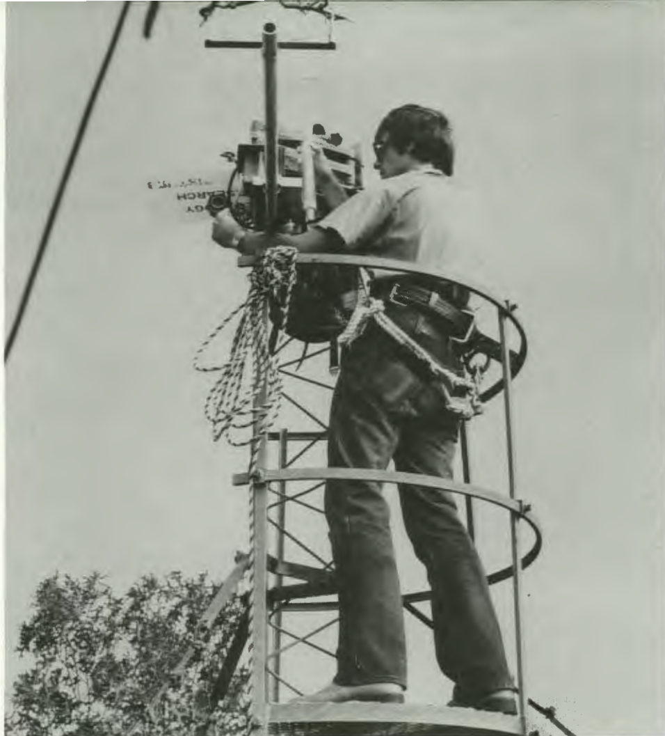
High on a tower in the Walker Branch Watershed in ORNL's National Environmental Research Park, Steve Lindberg calibrates an air sampler used to collect acidic particles in the atmosphere. The two Petri dishes extending laterally are dry deposition samplers that catch the kind of particles that settle on the forest canopy. This work is being done for the Electric Power Research Institute as well as DOE.
