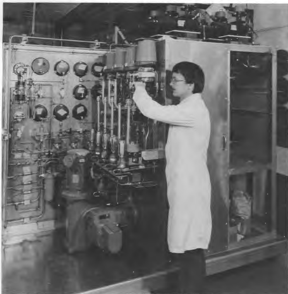
Jim Wilson works at the portable viscometer, which measures the physical properties of the black gummy product of a vacuum distillation column in one of DOE's coal conversion pilot plants. The unique capability of the device is that it measures the viscosity of residues containing a high loading of solids. It can be transported for use at pilot plants.
