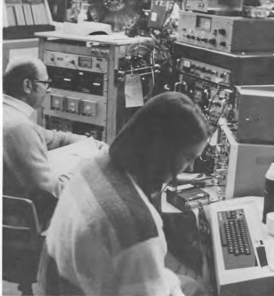
Manfred Krause works at the electron spectrometer in Wisconsin with Professor P. R. Woodruff of the University of Aberdeen, Scotland. The instrument, developed and built at ORNL and first used in February 1981, is part of a collaborative program with University of Wisconsin Professor Jim Taylor at the Synchrotron Radiation Center in Stoughton.
