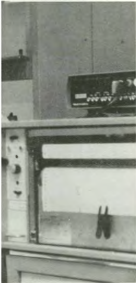
Charlie Coley, technician, rests a sample of PCB-contaminated oil on a gas chromatograph equipped with an electron capture detector. This apparatus is used to identify and quantify polychlorinated biphenyls in waste oil, spilled oil, and oils used as dielectric fluids in ORNL transformers. Looking on is Hershel Davis, who played an important role in re-establishing the method now used for PCB analysis in oils.
