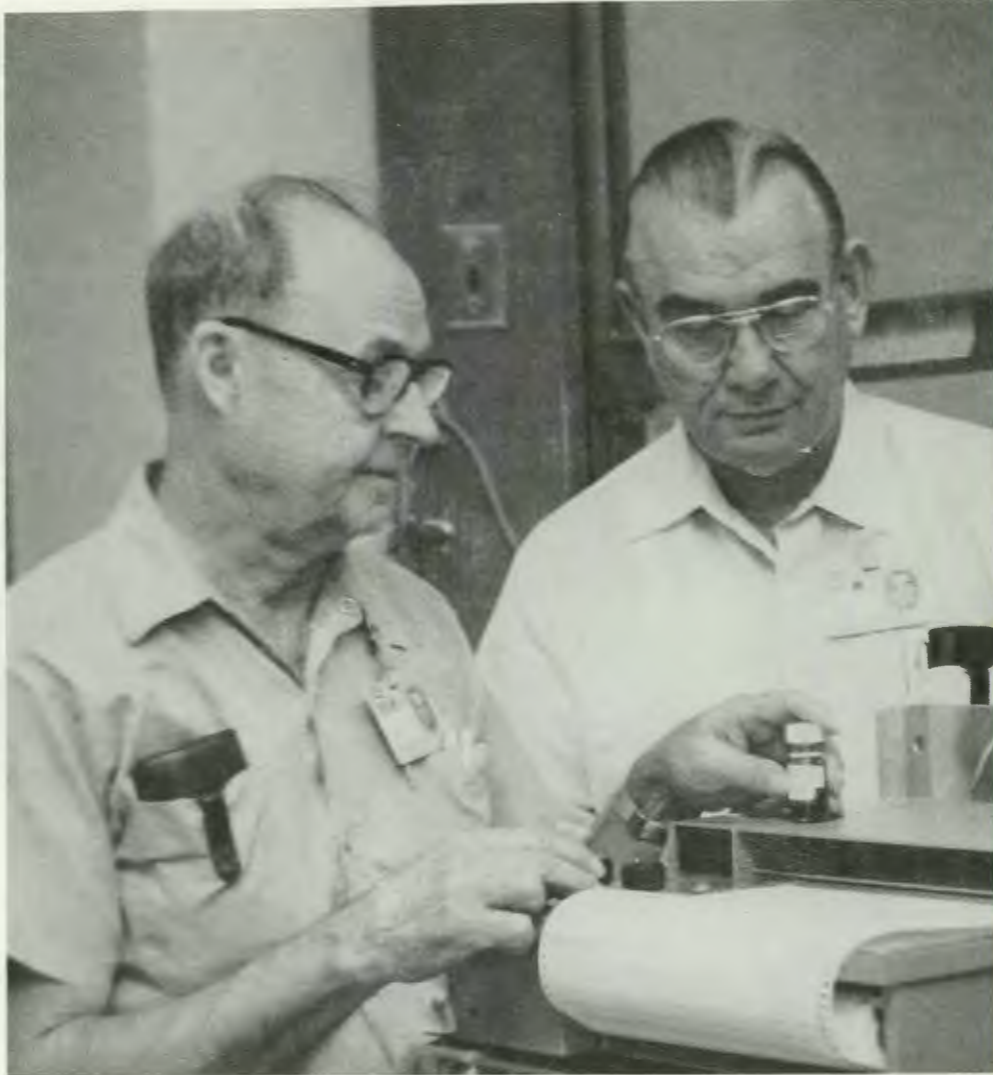
Kaye Webb and Fred Rogers check peaks in a book of oil profiles. The profiles, used in ORNL's oil identification program, were made at ORNL by running samples of the 40 different oils in ORNL's inventory through a gas chromatograph. By comparing the profile of an oil found as a visible sheen in ORNL waterways with the book profiles, analytical chemists can determine whether ORNL is responsible for the oil spill.
