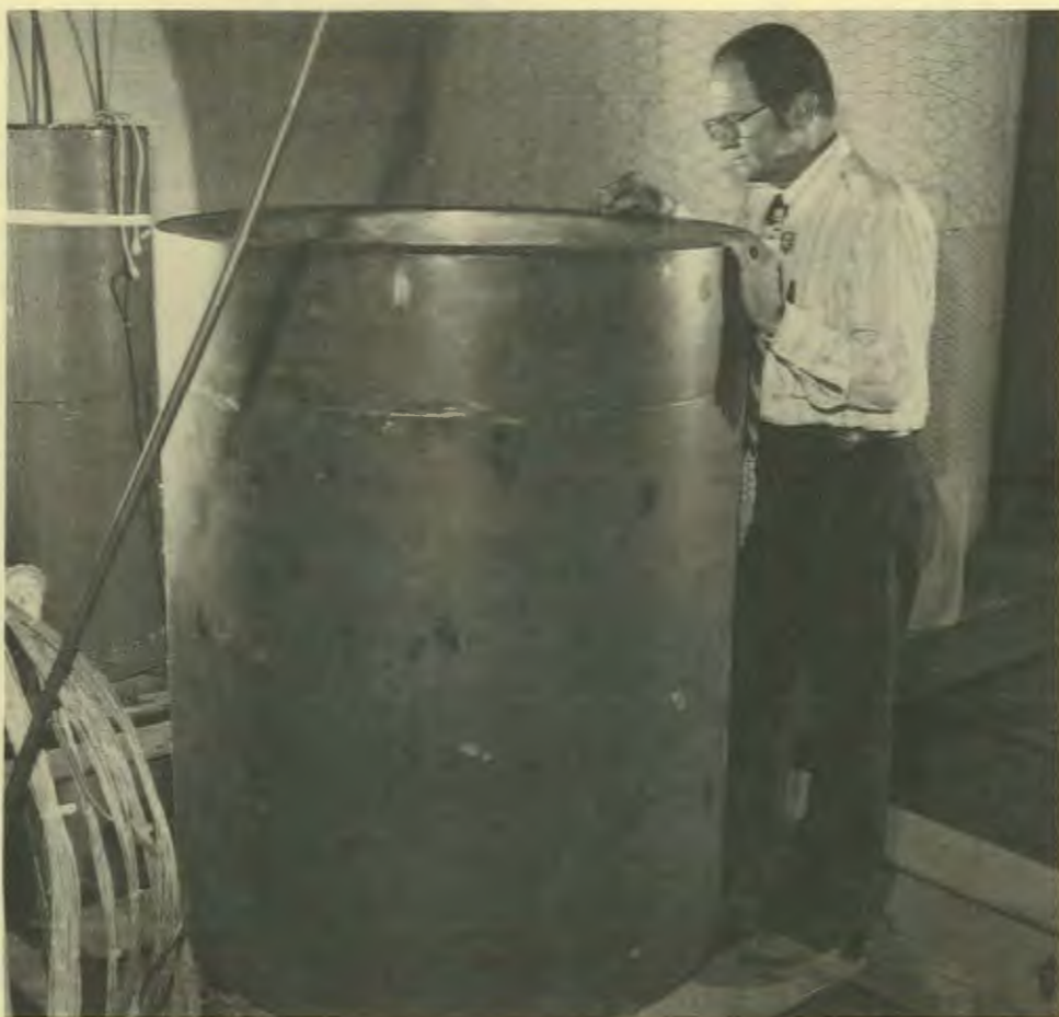
3900 kg test cylinder for TSE-5A being inspected by Sam Bolt prior to installation of instrumentation.
