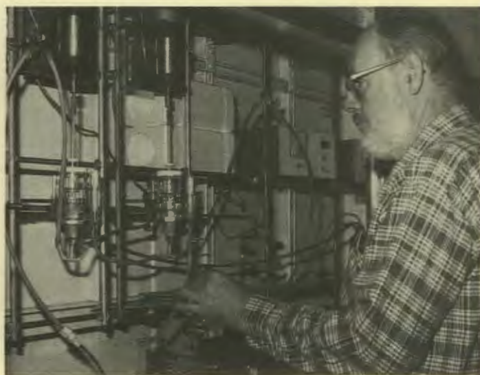
Dave McWhirter adjusts a solvent extraction technique that uses much less energy than a conventional distillation process in separating ethanol from water in the fermentation brew.
