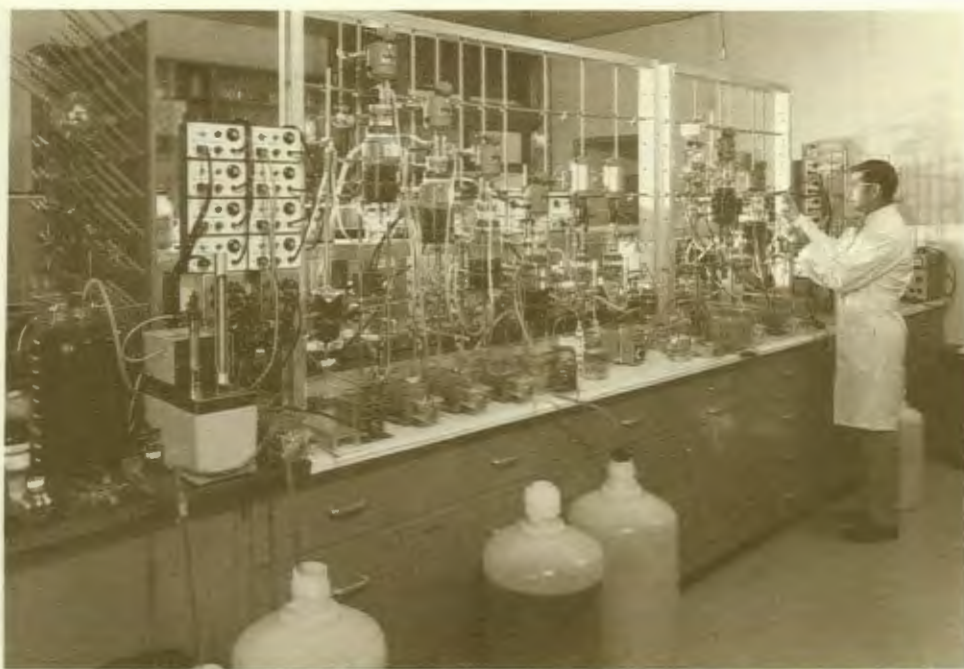
Fred Hurst works in the laboratory where members of the Chemistry and Chemical Technology divisions developed the DEPA-TOPO process for extracting uranium during production of phosphoric acid.
