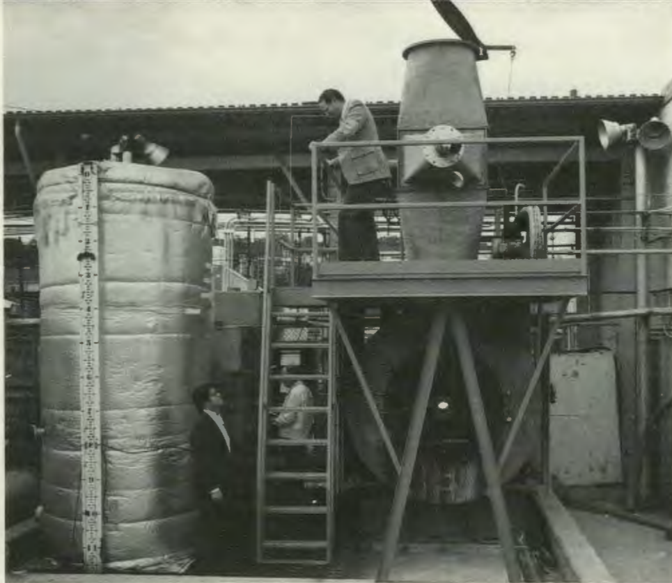
Vic Tennery (at top) and George Wei discuss the operation of the Ceramic Recuperator Analysis Facility. Recuperators are heat exchangers designed to recover heat from hot flue gases for preheating combustion air or gases low in energy content. ORNL is studying the potential of using recuperators made of ceramic materials for cutting consumption of fossil fuels by industry.
