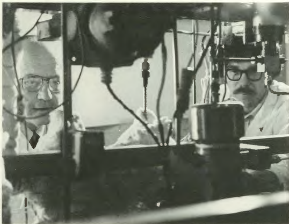
George Oswald (right) and Lloyd Youngblood adjust valves on the Coal Liquids Flow System at the Chemical Technology Division's Coal Conversion Facility. This system is being used to study the liquefaction of coal by slurry dissolution, similar to the Solvent Refined Coal (SRC) process now being tested in pilot plants in Alabama and Washington. ORNL researchers are studying the physical properties of coal liquids at temperatures and pressures typical of those at the SRC pilot plants. Information they obtain on viscosity, density, heat capacity, and thermal conductivity will aid engineers in designing SRC demonstration plants expected to be constructed in the 1980s under the supervision of DOE's Oak Ridge Operations.
